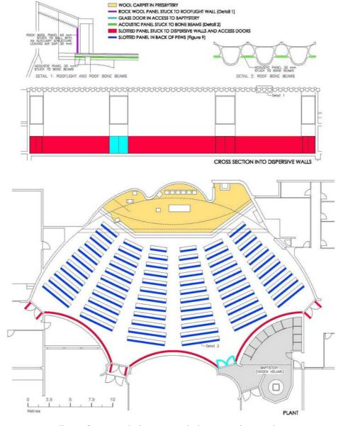
Fig. 8. Section and plan: proposed placement of materials.
