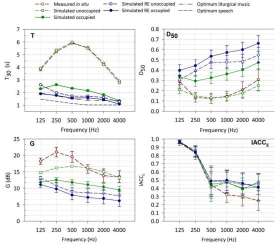
Fig. 11. Frequency behaviour of some spatially averaged acoustic parameters  $(T_{30}, D_{50}, G \text{ and } IACC_E)$ , corresponding to the measurement *in situ*, simulation of the current state and acoustic rehabilitation proposal (Source 1).
