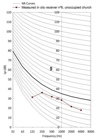
Fig. 6. NR curves and background noise spectrum recorded.
