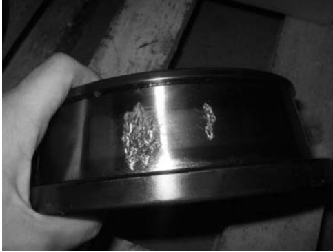
Fig. 16. Spalled inner race of a wind turbine.
