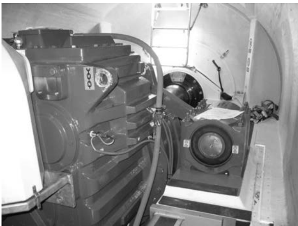
Fig. 3. View of the 1.5 MW wind turbine gearbox (front) and the main bearing (behind).
