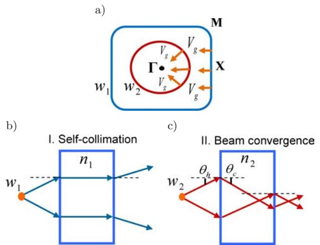
Fig. 6. a) Group velocity vectors on the second band EFCs. Wave frequencies and refraction indexes satisfy  $w_2 > w_1$  and  $0 > n_2 > n_1$ , b) a ray-trace representation of the self-collimation effect, c) a ray-trace representation of the beam convergence effect.
