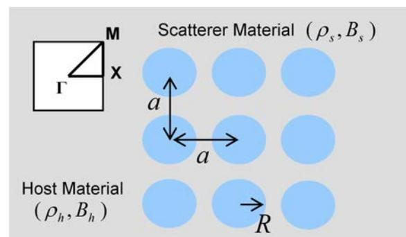
Fig. 1. The square lattice sonic crystal structure and related parameters.
