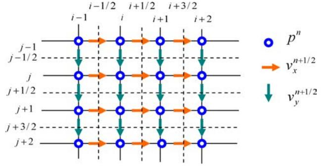
Fig. 3. Spatial sampling points for the two-dimensional FDTD method.
