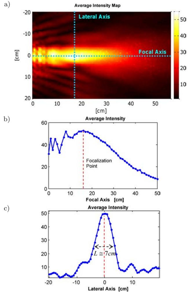
Fig. 8. Intensity map (a) obtained for the experimental sonic crystal slab at 9900 Hz, intensity versus-focal axis plots (b) and intensity versus-lateral axis (c).
