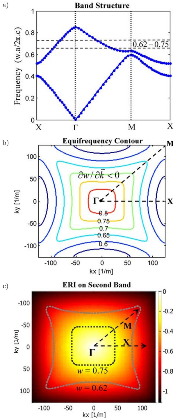
Fig. 5. Band structure in (a), EFC in (b) and ERI in (c) of the second frequency band for the squared lattice sonic crystal. Lattice constant  $a = 25$  mm, scatterer radius  $r = 10$  mm, filling ratio  $f_r = 0.50$  and speed of sound  $c_h = 340$  m/sn.
