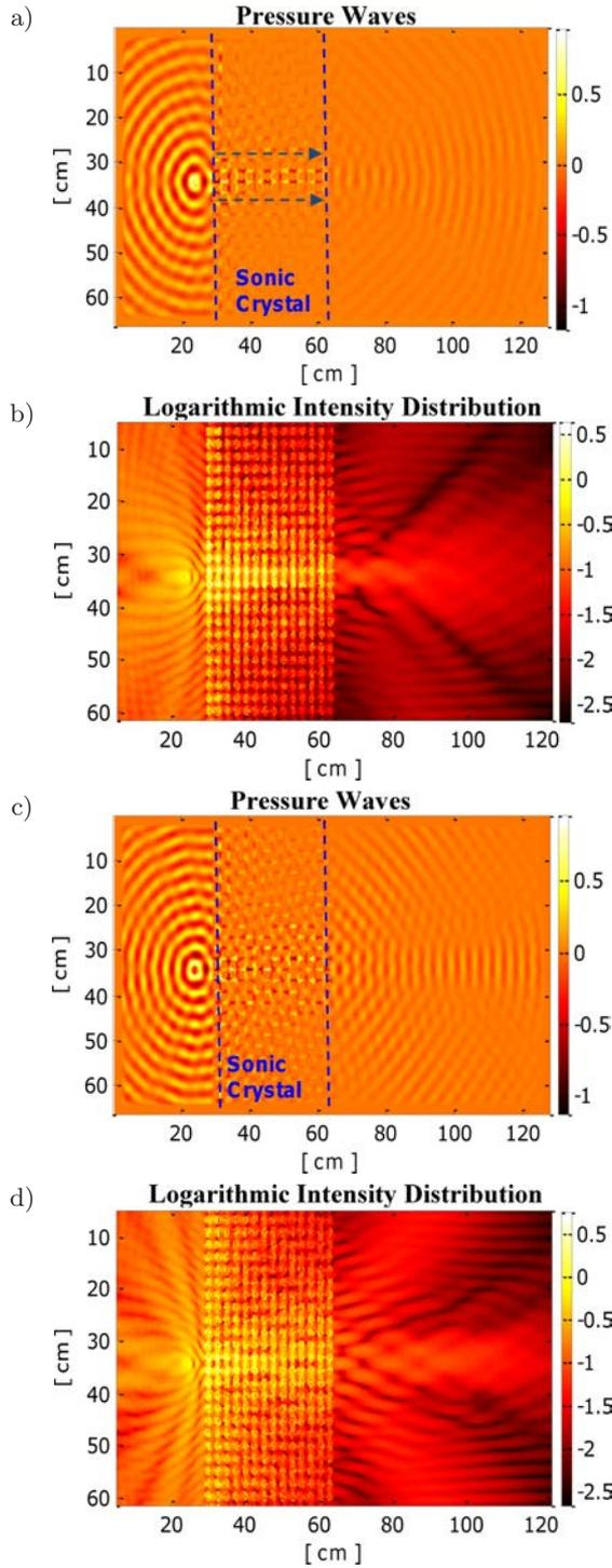
Fig. 7. The pressure field pattern ( $p$ ) in (a) and (c) and the logarithmic intensity distribution ( $\log_{10}(p^2)$ ) in (b) and (d) from the FDTD simulation. Lattice constant  $a = 25$  mm, scatterer radius  $r = 10$  mm, filling ratio  $f_r = 0.50$  and speed of sound  $c_h = 340$  m/sn. Frequency of wave source is 9200 Hz in (a)–(b) and 9900 Hz in (c)–(d).
