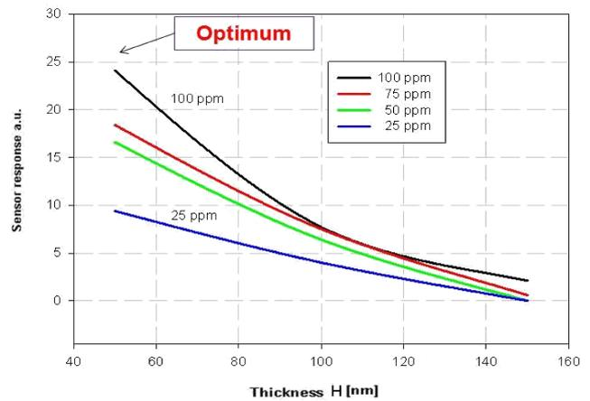
Fig. 6. Influence of the thickness of the  $\text{WO}_3$  layer on the response of carbon monoxide vs. concentration: 25, 50, 75, 100 ppm) in  $T = 40^\circ\text{C}$ .
