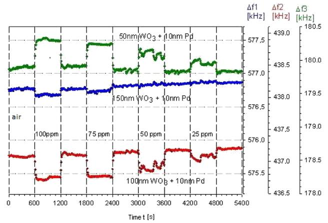
Fig. 4. Experimental results – response ( $\Delta f$ ) sensor for thickness layers of the  $\text{WO}_3 + \text{Pd}$ : 50, 100, 150 nm CO gas (25, 50, 75, 100 ppm),  $T = 40^\circ\text{C}$ .
