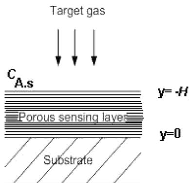
Fig. 1. Thin semiconducting layer on a piezoelectric substrate (HEJCZYK, URBAŃCZYK, 2013).
