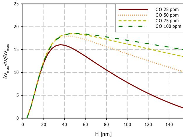
Fig. 3. Relative changes of velocity vs. sensor layer thickness – numerical results. Sensitivity coefficient  $a = 0.5 \text{ ppm}^{-1}$ ,  $\sigma_S = 4.7 \times 10^{-7}$ ,  $k = 10^8 \text{ s}^{-1}$ ,  $D_K = 10^{12} \text{ nm}^2 \text{ s}^{-1}$ ,  $E_g = 2.7 \text{ eV}$ ,  $M = 28 \text{ g/mol}$  (CO) (HEJCZYK, URBAŃCZYK, 2013).
