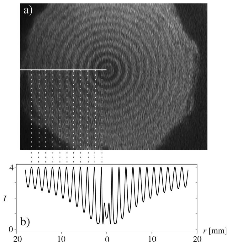
Fig. 2. Virtual image of the reconstructed hologram (a). Theoretical cross-section of the light intensity of the reconstructed hologram (b).
