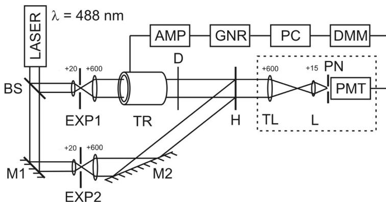
Fig. 1. The experimental set-up. BS – beamsplitter; EXP1, EXP2 – expanders in the object and reference beams, respectively; M1, M2 – mirrors; TR – cylindrical transducer; D – diffuser; H – holographic plate; TL – transforming lens; L – lens; PN – pinhole; PMT – photomultiplier; DMM – digital multimeter; PC – computer; GNR – synthesizer/function generator; AMP – power amplifier.
