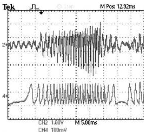
Fig. 3. Beat frequency signal registered by a microphone (top) and optical detector (bottom – see the triangle-like shape).
