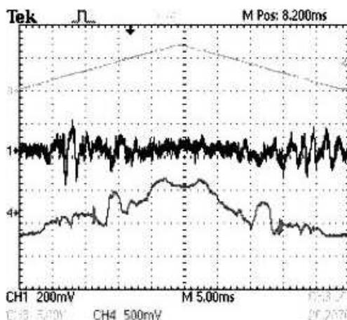
Fig. 4. Driven signal on a vibration exciter (top), signature registered by a microphone (center) and optical detector (bottom).
