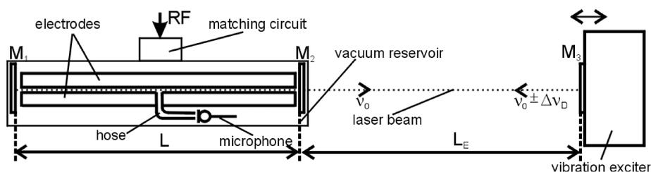
Fig. 2. Experimental setup.  $\nu_0$  – frequency of the output laser radiation,  $\Delta\nu_D$  – Doppler shift.
