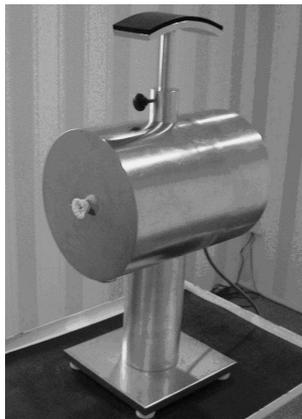
Fig. 1. The acoustic test fixture worked out for insertion loss measurements of ear-plugs [2].
