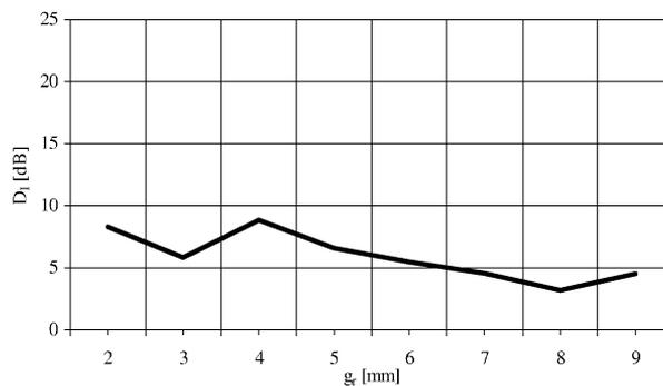
Fig. 6. Acoustic insulation  $D_I$  vs. acoustic insulation lining thickness  $g_r$ ,  $f_{\text{okt}} = 250$  [Hz].
