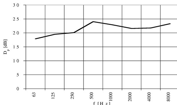
Fig. 1. Acoustic insulation crane's cabin – result of measurements (octave band) [4].
