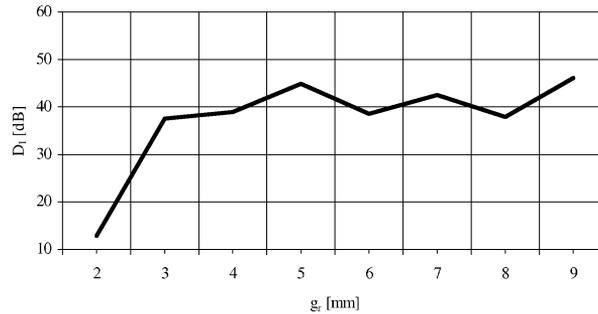
Fig. 8. Acoustic insulation  $D_I$  vs. acoustic insulation lining thickness  $g_r$ ;  $f_{\text{okt}} = 1000$  [Hz].
