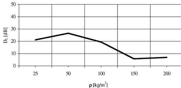
Fig. 7. Acoustic insulation  $D_I$  vs. mineral wool density  $\rho$ ,  $f_{\text{okt}} = 250$  [Hz].
