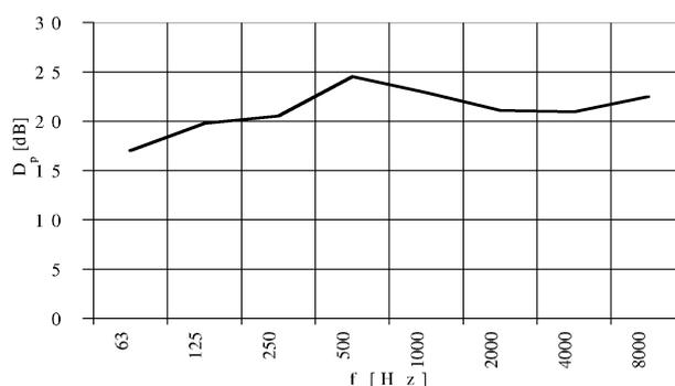
Fig. 2. Acoustic insulation of the front wall – determined from measurements (octave band) [4].
