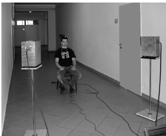
Fig. 2. The measurement (and listening) set-up in environment 3 – building corridor.
