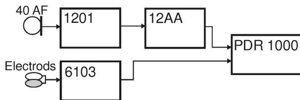
Fig. 3. The block diagram of the measurement setup, where: 40 AF – the measuring microphone, G.R.A.S; 12AA – the microphone preamplifier, G.R.A.S; 6103 – the electroglottograph (EGG), KAYELEMETRICS; PDR 1000 – digital magnetic recorder, HHB.
