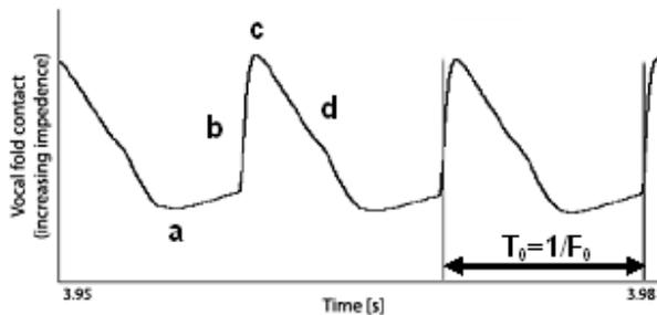
Fig. 2. Time dependence of the EGG signal – glottogram.
