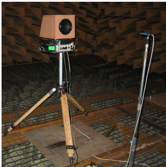
Fig. 2. The station for directional characteristics' measurement of Visaton BG17 loudspeaker in closed box enclosure.
