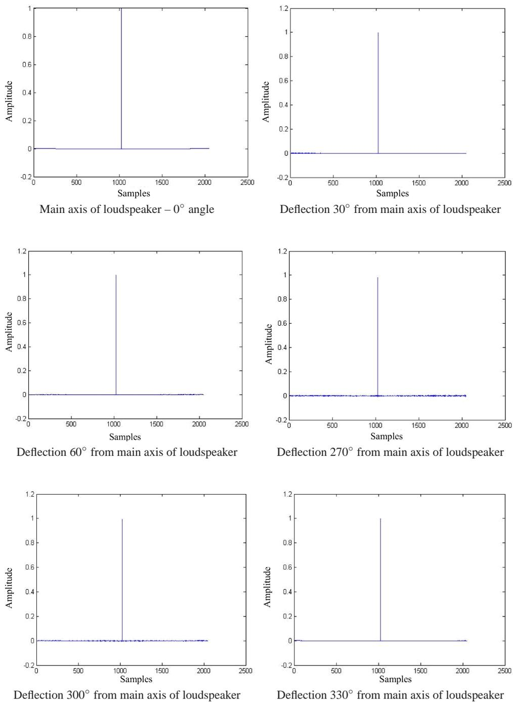
Fig. 6. Impulse responses of BG17 loudspeaker in closed box enclosure after correction with digital inverse equalizer.
