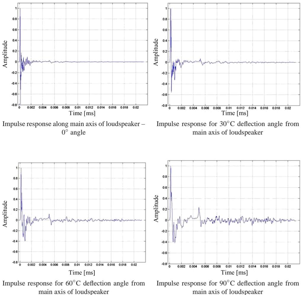
Fig. 4. Impulse responses of BG17 loudspeaker in enclosure, determined for various angles within horizontal and vertical planes.
