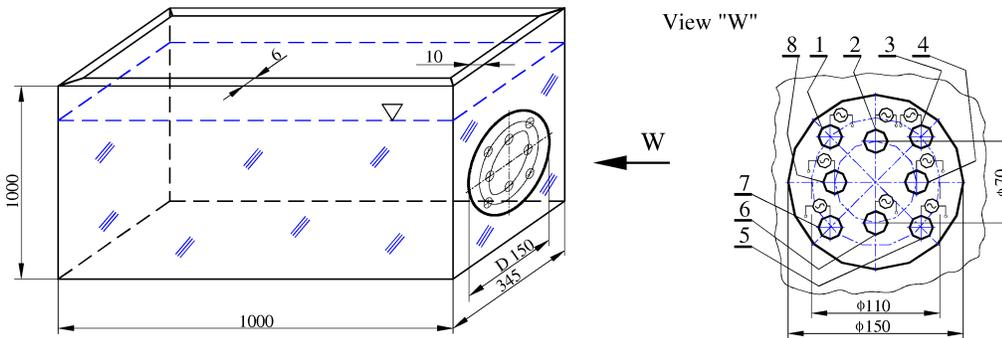
Fig. 1. Geometry of aquarium (1, 3, 5, 7 piezoelements type 1, thickness  $h_1 = 0.28$  mm, 2, 4, 6, 8 piezoelements type 1, thickness  $h_2 = 0.21$  mm, marked: A2, A4, A6, A8).
