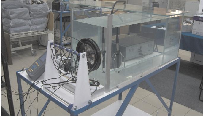
Fig. 3. The view of experimental aquarium and plate with piezoelements.
