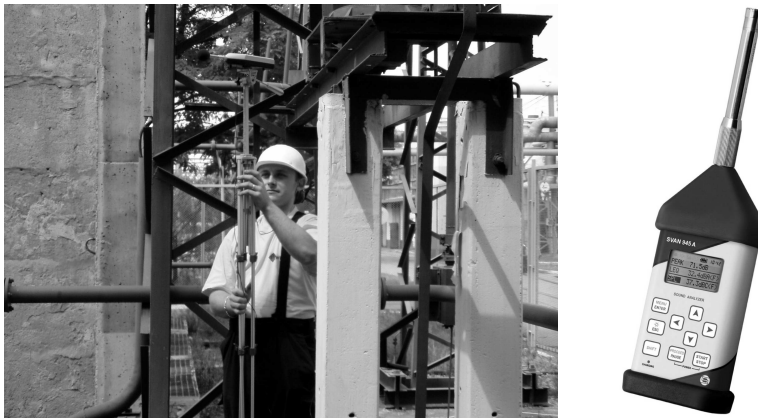
Fig. 1. Measuring appliance (SVAN 945A) used for measurements at the electric power station.
