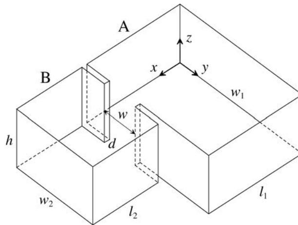
Fig. 1. Irregularly shaped enclosure consisting of two connected rectangular subrooms denoted by A and B.
