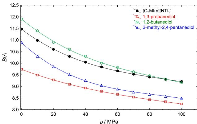
Fig. 3. Dependence of the nonlinear parameter  $B/A$  on pressure  $p$  at temperature 298.15 K for: •  $[C_2MIm][NTf_2]$ , this work; □ 1,3-propanediol (ZORĘBSKI, ZORĘBSKI, 2014); ○ 1,2-butanediol (ZORĘBSKI, ZORĘBSKI, 2014); and △ 2-methyl-2,4-pentanediol (ZORĘBSKI, ZORĘBSKI, 2014). Lines – arbitrary, to aid the eye.
