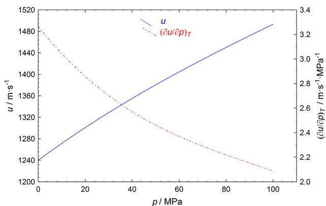
Fig. 2. Dependence of the speed of sound  $u$  (continuous line) and the pressure derivative of the speed of sound  $(\partial u / \partial p)_T$  (dashed line) on pressure  $p$  for  $[\text{C}_2\text{MIm}][\text{NTf}_2]$  at temperature 298.15 K. Lines are obtained from smoothing equation  $u = u(p, T)$  reported in (DZIDA *et al.*, 2013) and from derivation of this smoothing equation.
