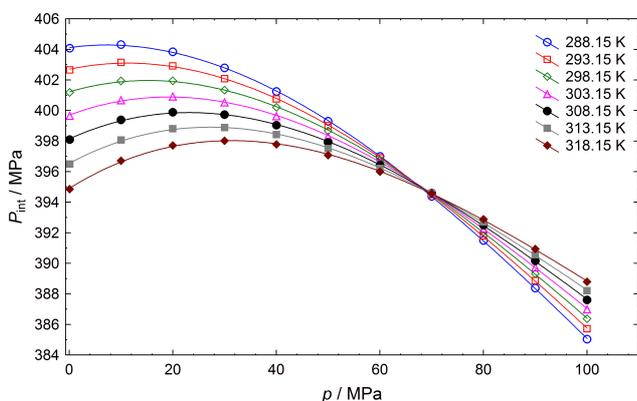
Fig. 4. Isotherms of the dependence of the internal pressure  $P_{\text{int}}$  on pressure  $p$  at temperatures in the range 288.15–318.5 K with the 5 K step for  $[\text{C}_2\text{MIm}][\text{NTf}_2]$ . Lines – third order polynomials.
