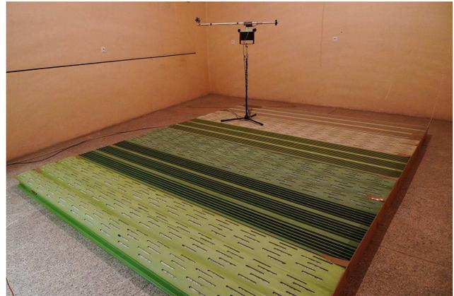
Fig. 9. A sample consisting of alternate panels: a perforated Schroeder diffuser and a perforated cylindrical profile.
