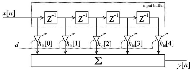
Fig. 3. General VFD filter structure applied to SRC.
