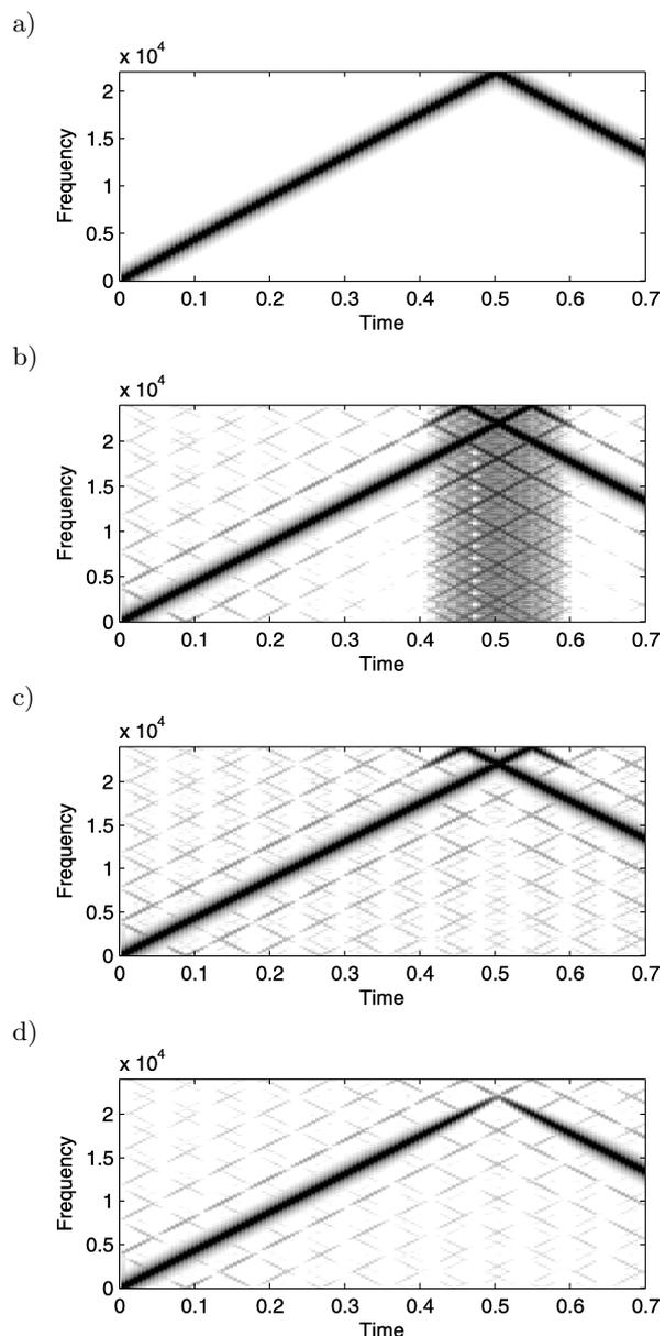
Fig. 6. Spectrograms illustrating resampling with constant resampling ratio 160/147 using VFD filters from Fig. 5 implemented with the Farrow structure of order  $q = 5$ : a) input chirp signal, b) signal resampled using minimax FD filters ( $f_a = 0.4$ ), c) signal resampled using fullband ( $f_c = 0.5$ ) FD filters designed using offset window, d) signal resampled using FD filters designed using offset window for  $f_c = f_a$ .
