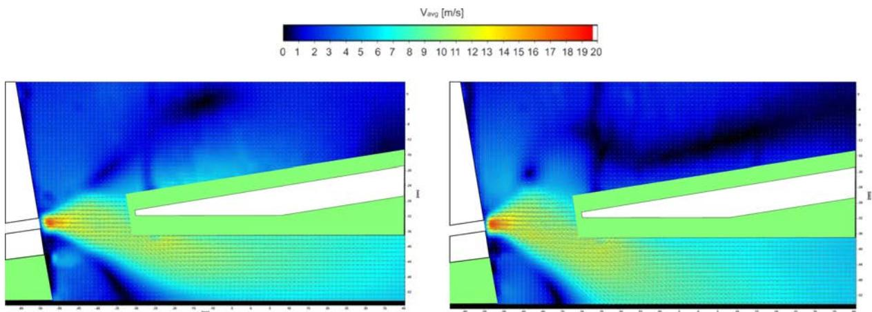
Fig. 7. Mean flow velocity field at 13 m/s (left) and 16 m/s (right).
