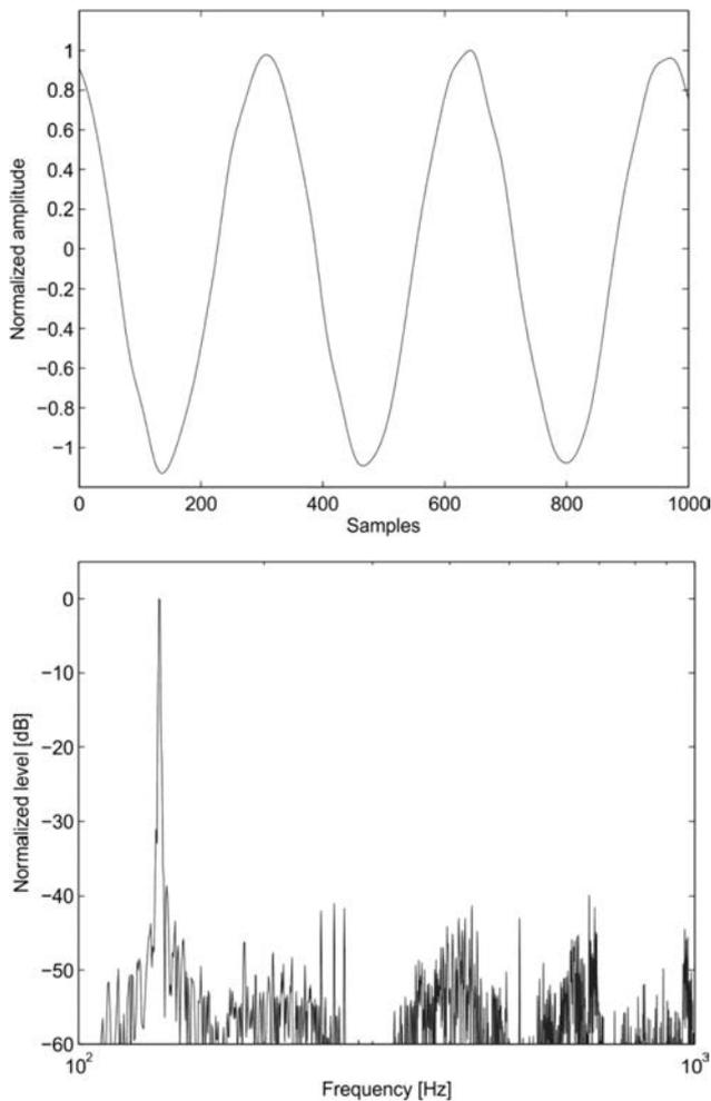
Fig. 3. The pressure signal generated by the pipe in time (top) and frequency (bottom) domains with normalized amplitudes.
