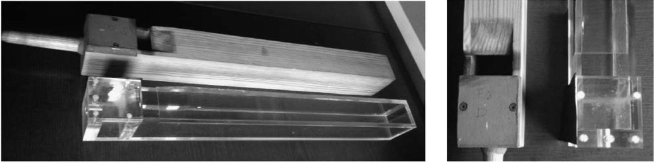
Fig. 1. The original wooden organ pipe and its transparent model (left) and the details of the pipe mouth and labium (right).
