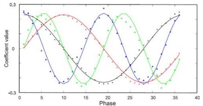
Fig. 10. POD first 4 temporal modes (coefficients  $a_k(n)$  in Eq. (2)) of measured data (stars and triangles) and perfect cosinusoidal harmonic components shifted in pairs by 90 degrees.
