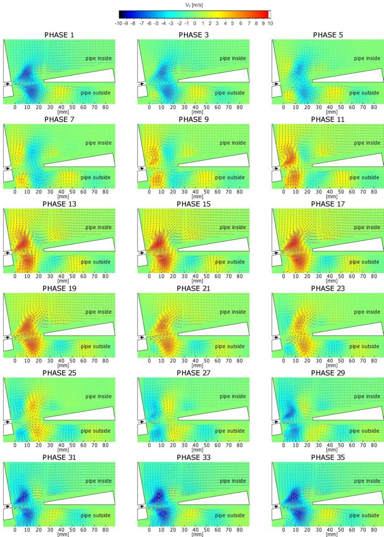
Fig. 11. The two POD modes approximation of an acoustic velocity field evolution in transparent pipe model (fundamental frequency of 128 Hz, one period divided into 36 equidistant phases, every second phase is shown).
