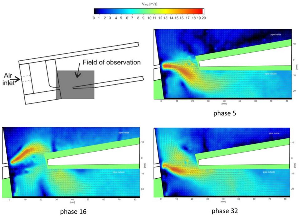
Fig. 6. Flow field evolution in chosen phases in the transparent Plexiglas pipe model.
