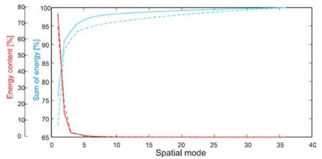
Fig. 8. Vibrating energy distribution in POD modes for two air inlet velocity cases.
