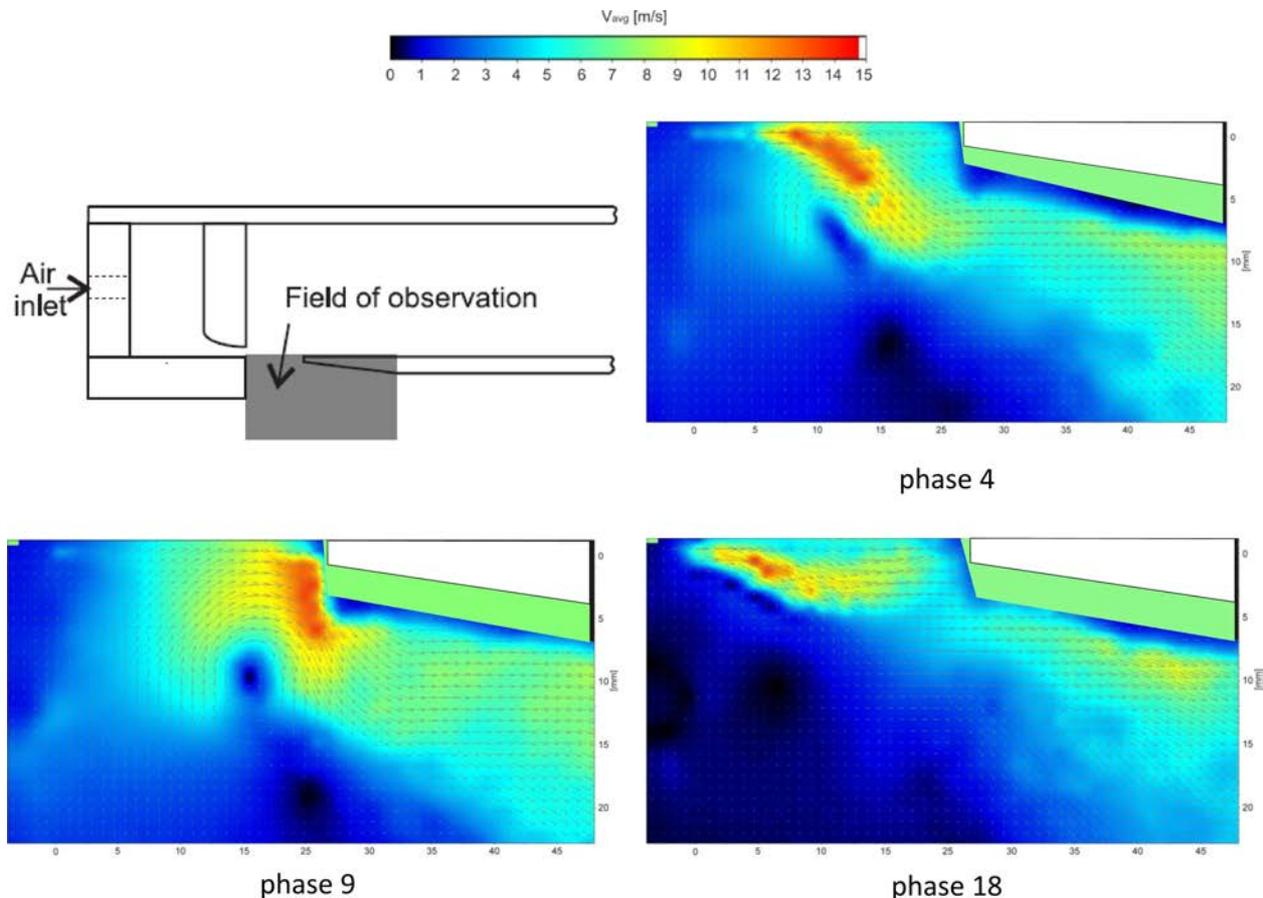
Fig. 5. Flow field evolution in chosen phases in the original organ pipe.
