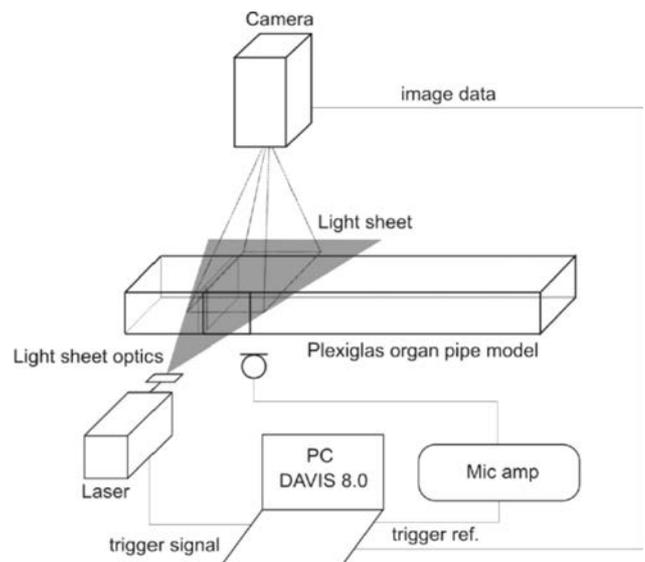
Fig. 4. Schematic diagram of the experimental stand.
