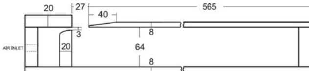
Fig. 2. Dimensions (in mm) and geometrical details of the Plexiglas pipe model.
