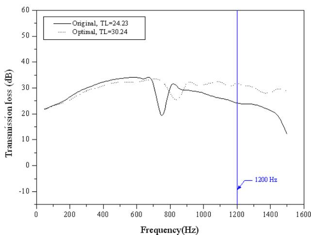
Fig. 19. TL curves with/without optimisation at target 1200 Hz [case II: three-chamber plenum partitioned with sound-absorbing and centre-opening baffles ( $\alpha = 0.83$ )].
