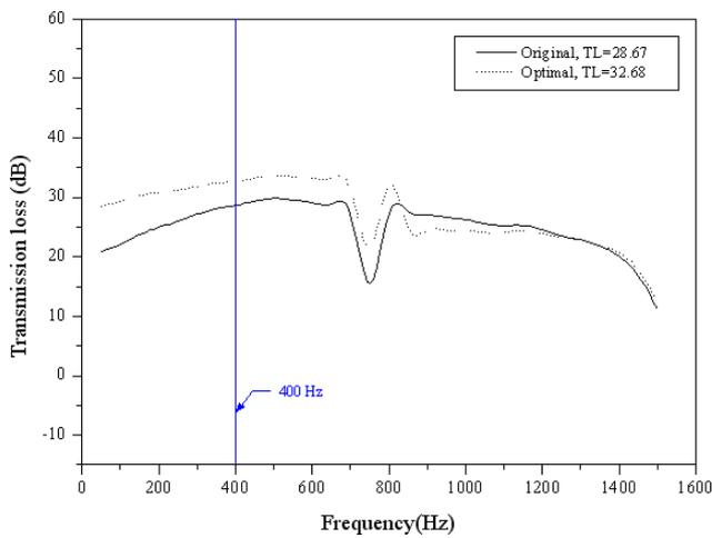
Fig. 11. TL curves with/without optimisation at target 400 Hz [case I: two-chamber plenum partitioned with sound-absorbing and centre-opening baffles ( $\alpha = 0.83$ )].
