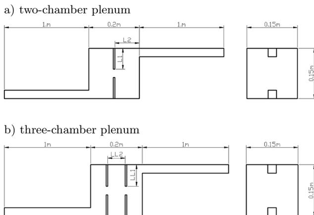
Fig. 1. Dimensions for two kinds of multi-chamber plenums: a) a two-chamber plenum partitioned with a centre-opening baffle; b) a three-chamber plenum partitioned with two centre-opening baffles.
