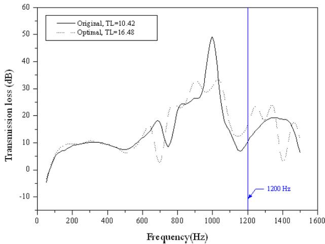
Fig. 10. TL curves with/without optimisation at target 1200 Hz [case I: two-chamber plenum partitioned with non-sound-absorbing and centre-opening baffles ( $\alpha=0.1$ )].
