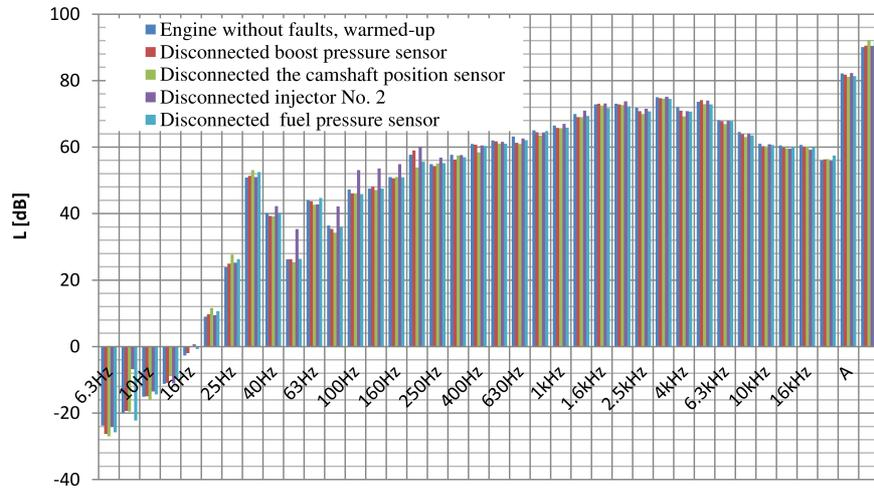
Fig. 2. Graph of the average sound pressure level  $L_{mA}$  for the speed of 1,000 rpm.
