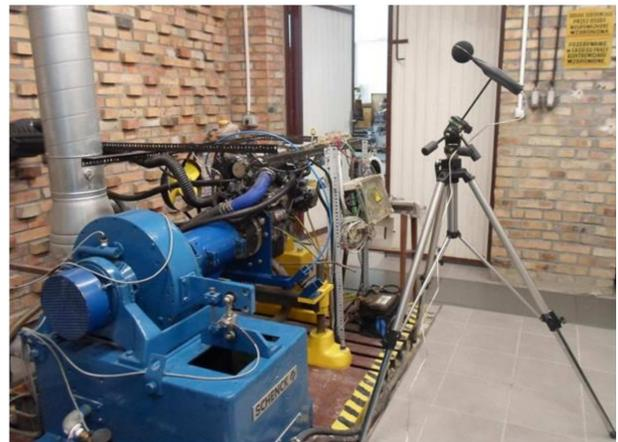
Fig. 1. Test rig for acoustic measurements.
