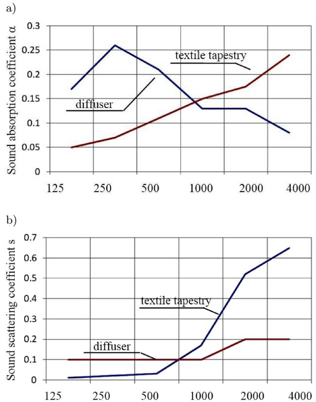
Fig. 11. Acoustic parameters of the textile tapestry and the diffuser of Fig. 9 used in computer simulation (octave resolution, frequency range 125–4000 Hz): a) sound absorption coefficient  $\alpha$ , b) sound scattering coefficient  $s$  (KAMISIŃSKI *et al.*, 2012b).
