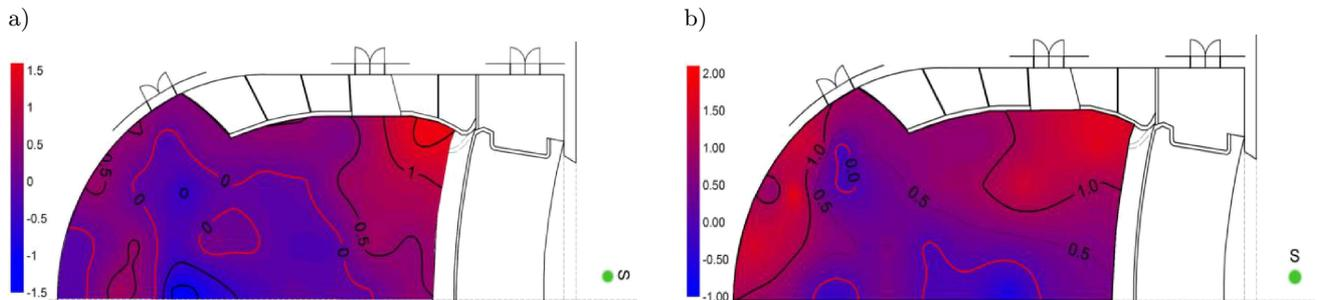
Fig. 14. The effect of mounting the diffusers on the sound strength  $G$  in octave bands: (a) 0.5–1 kHz and (b) 4 kHz.
