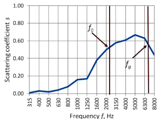
Fig. 10. The sound scattering coefficient  $s$  for the diffuser of Fig. 9 obtained from acoustics measurements (third-octave resolution, frequency range 314–8000 Hz).  $f_0$  and  $f_g$  are the lower and the higher sound diffusion limiting frequencies, respectively. It is assumed that sound diffusion occurs at frequencies above  $0.5 f_0$  (KAMISIŃSKI *et al.*, 2012b).
