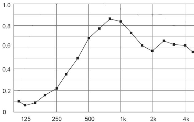
Fig. 24. The sound absorption frequency characteristic for the microperforated foil stretched at a distance of 10 cm from glass pane. Film parameters: thickness 0.18 mm; 500,000  $\varnothing 0.1$  mm holes per m<sup>2</sup>; perforation rate 1%; sound absorptivity class D,  $\alpha_w = 0.55$  (NOCKE, 2014).
