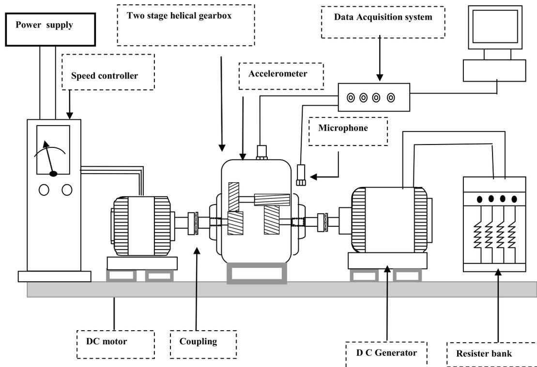
Fig. 1. Experimental setup of two stage helical gearbox.
