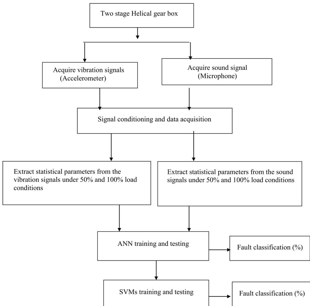
Fig. 5. Flow chart of gear fault diagnostic procedure.
