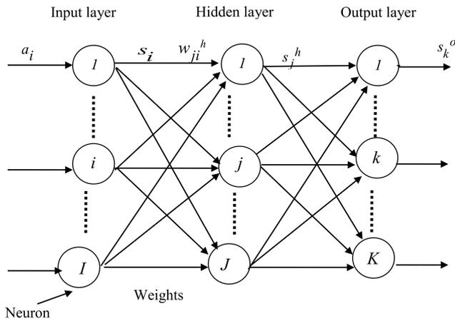
Fig. 8. Three layered feed forward neural network.
