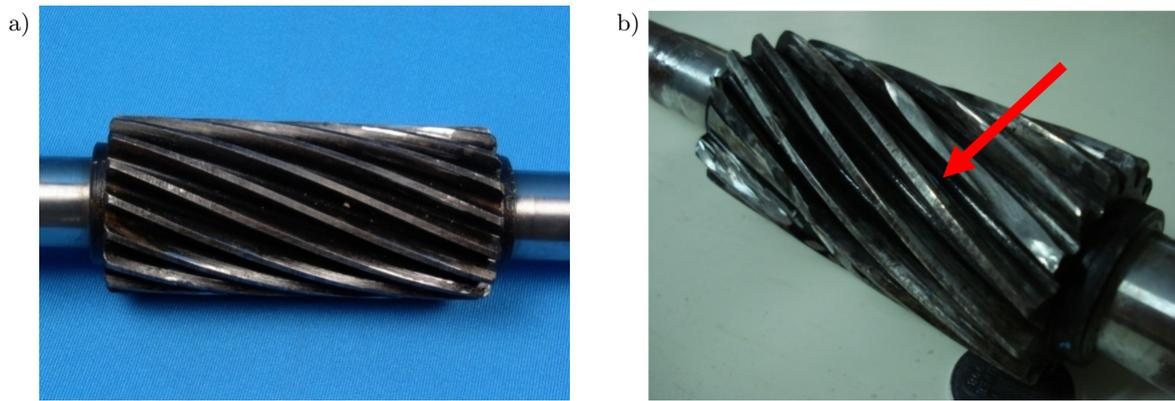
Fig. 4. Test pinions: a) healthy pinion, b) defective pinion.
