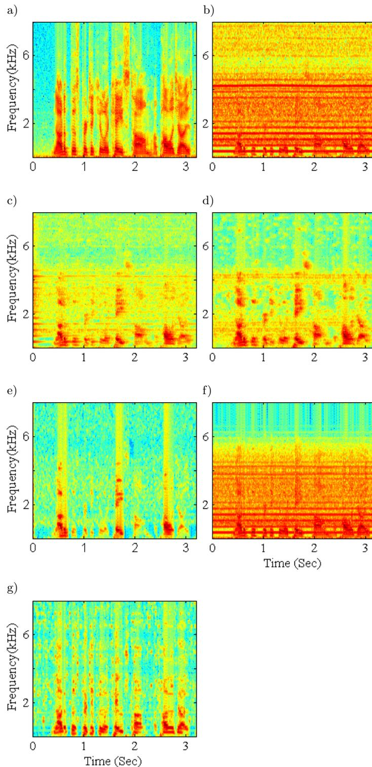
Fig. 8. Spectrums of (a) clean speech, (b) noisy speech with factory background noise (SNR = -5 dB), and enhanced speech by applying five algorithms, including (c) MMSE84, (d) MMSE04, (e) Wiener96, (f) BTW, and (g) WPT-MTEO, respectively.
