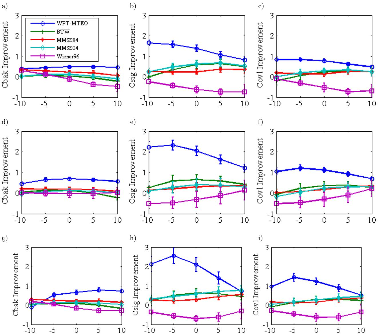
Fig. 7. Improvements of  $C_{bak}$ ,  $C_{sig}$ , and  $C_{ovl}$  obtained from 30 noisy speech signals with three different background noises (i.e., factory noise in (a), (b), (c), machine shop noise in (d), (e), (f), and station noise in (g), (h), (i)) applied five speech enhancement algorithms at various input SNRs ( $-10 \text{ dB} < \text{SNRs} < 10 \text{ dB}$ ).
