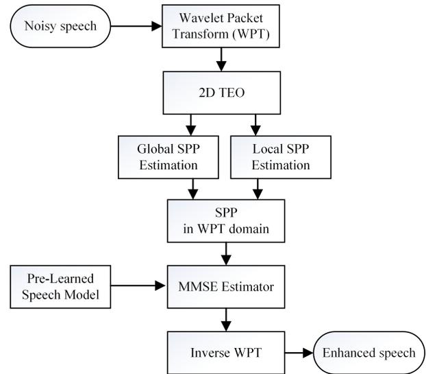
Fig. 5. The flow chart of implementation of the proposed algorithm.
