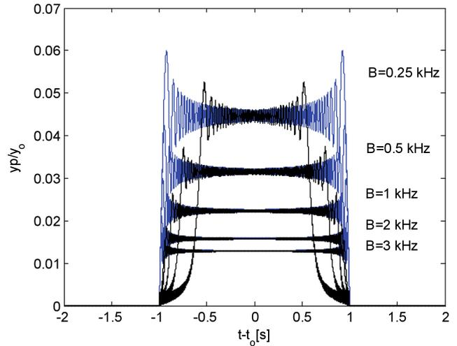
Fig. 14. LFM crosstalk signals at LFM filter output, blue line  $v = 0$  m/s, black line,  $v = 10$  m/s,  $T = 1$  s,  $f_0 = 15$  kHz.
