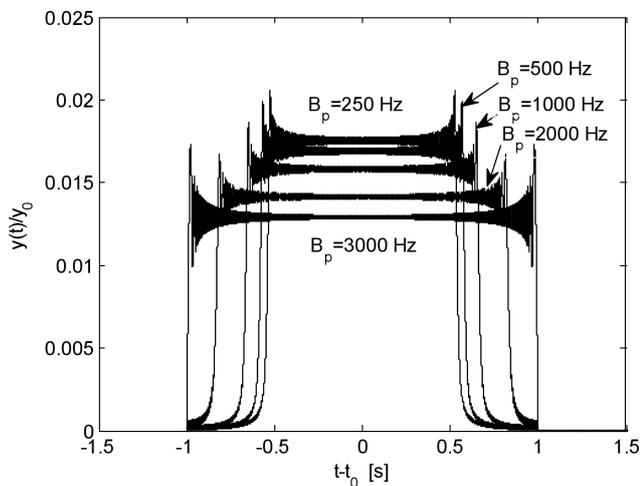
Fig. 11. LFM crosstalk signals at LFM filter output for opposite direction of frequency change,  $T = 1$  s,  $B = 3$  kHz.
