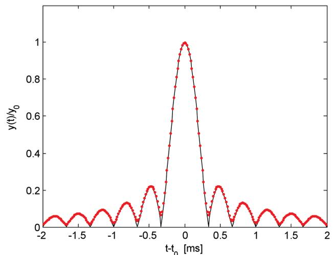
Fig. 3. Echo signals at matched receiver output for LFM (black line) and HFM signals (red line),  $B = 3$  kHz,  $T = 1$  s,  $t_o = 1$  s,  $y_o = 6 \cdot 10^4$ , the scale of the bottom chart has been enlarged.
