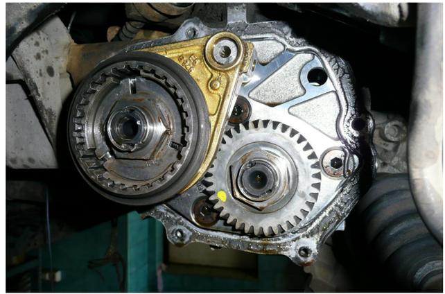
Fig. 1. The gear with denoted damaged tooth.
