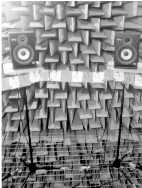
Fig. 2. The reproduction system for the stereo basis of 30^\circ . The sheets of paper marking the directions can be seen.
