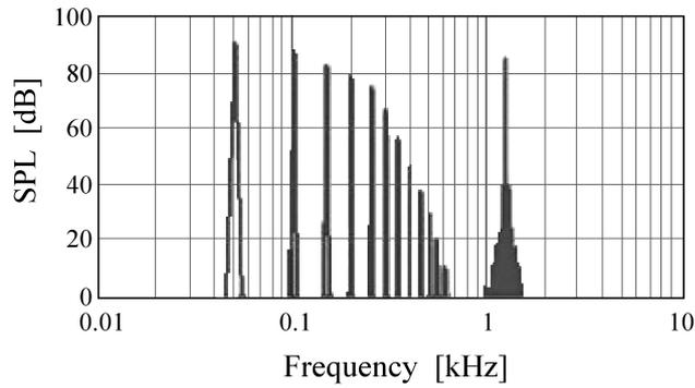
Fig. 12. Harmonic and intermodulation distortion produced by the system with nonlinear stiffness, depending on displacement according to Eq. (22). Excitation the same as in Fig. 10.
