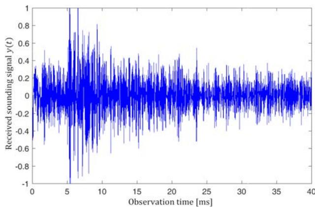
Fig. 9. A sequence of received pulses if the narrow signal pulse is transmitted with a period of transmitting of 40 ms.
