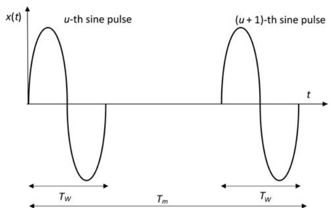
Fig. 1. A very short impulse (sounding signal) is transmitted periodically for measuring PDP of the shallow water channel.
