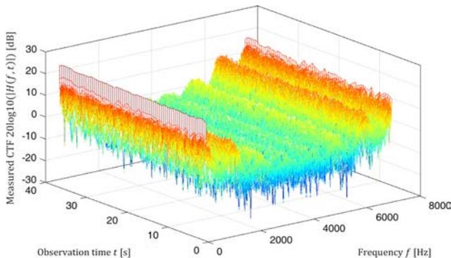
Fig. 7. The CTF of a static channel measured in Thonghat lake.
