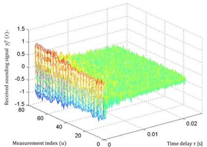
Fig. 5. The received sounding signal over a static underwater channel measured in Thongnhat lake.
