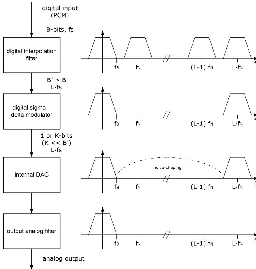
Fig. 1. Block diagram of a typical sigma-delta DAC.
