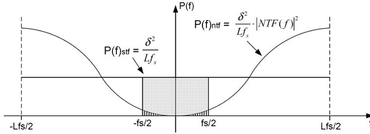
Fig. 3. Oversampling and noise shaping in sigma-delta modulator.
