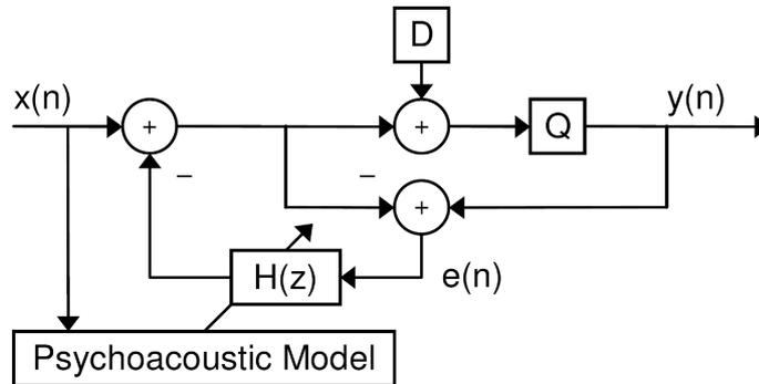
Fig. 13. Time-variant DSDM model with adaptive feedback filter  $H(z)$  controlled by a psychoacoustic model (HELMRICH *et al.*, 2007).
