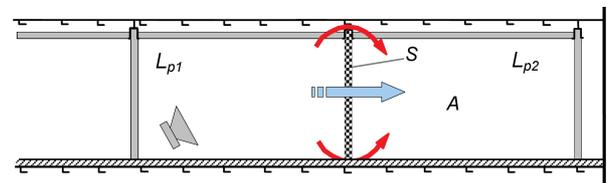
Fig. 3. Measurement method of bulkhead transmission loss.
