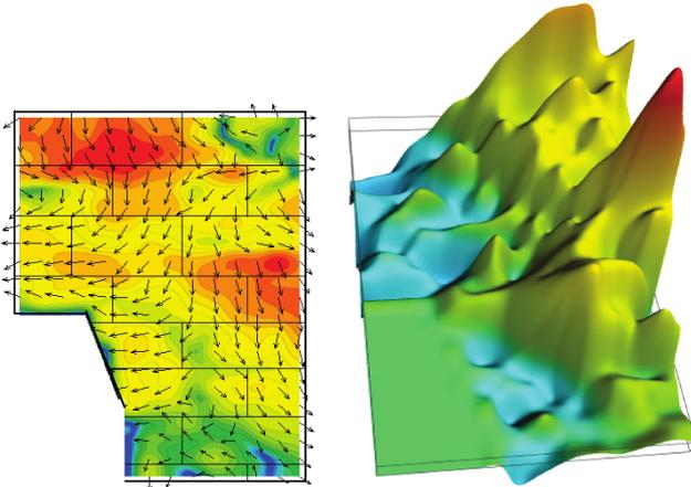
Fig. 9. Noise radiation into cabin from “floating floor”.
