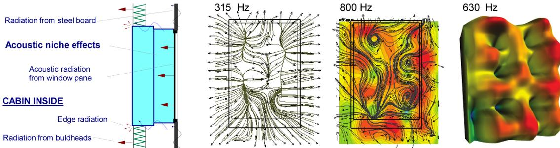
Fig. 7. Graphical form of visualization of acoustic radiation of the cabin windows.
