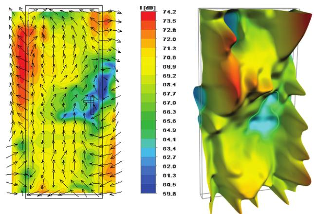
Fig. 8. Acoustic vectors field distribution close to the cabin door.
