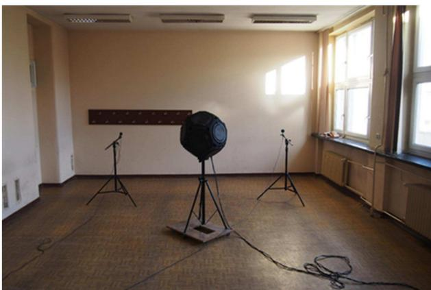
Fig. 2. View of the classroom during the measurement with an exemplary location of an omnidirectional loudspeaker and two measurement points.
