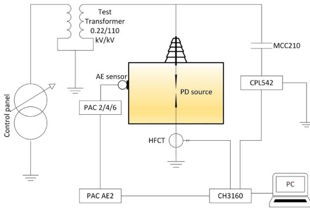
Fig. 1. Layout of the measuring set up.
