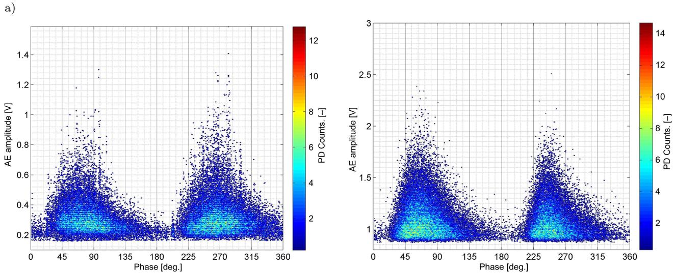
Fig. 7. Exemplary PRPD patterns achieved using AE method – amplitude criterion applied:
