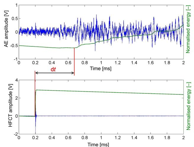
Fig. 2. Exemplary graphical layout of the DCA process using HFCT.
