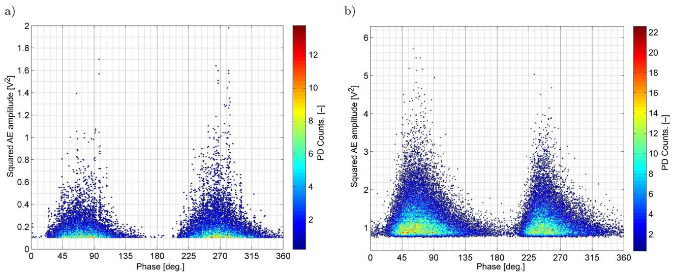
Fig. 8. Exemplary PRPD patterns achieved using the AE method – energy criterion applied:
