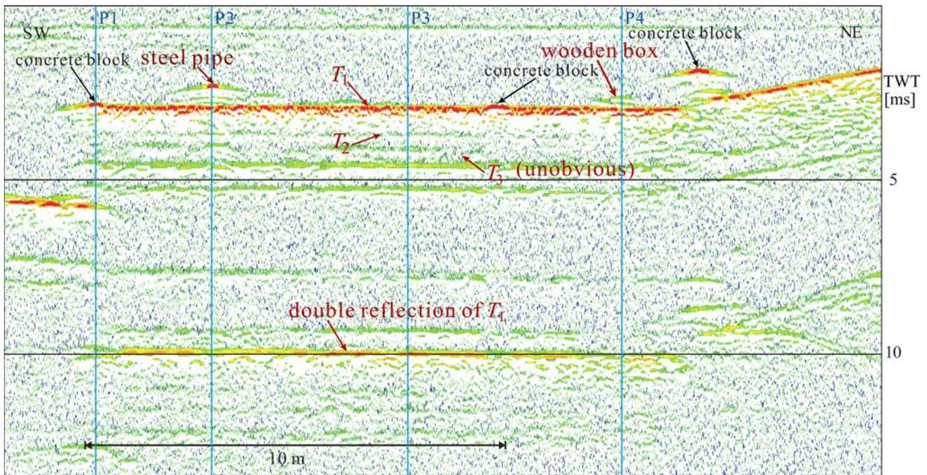
Fig. 5. Profile of the actual resolution experiment of SES-2000 SBP, frequency setting was 15 kHz, and PW setting was 67  $\mu$ s.  $T_1$  was the reflection event of water-bottom interface.  $T_2$  was the reflection event of sand-clay interface.  $T_3$  was the reflection event of clay-concrete interface.
