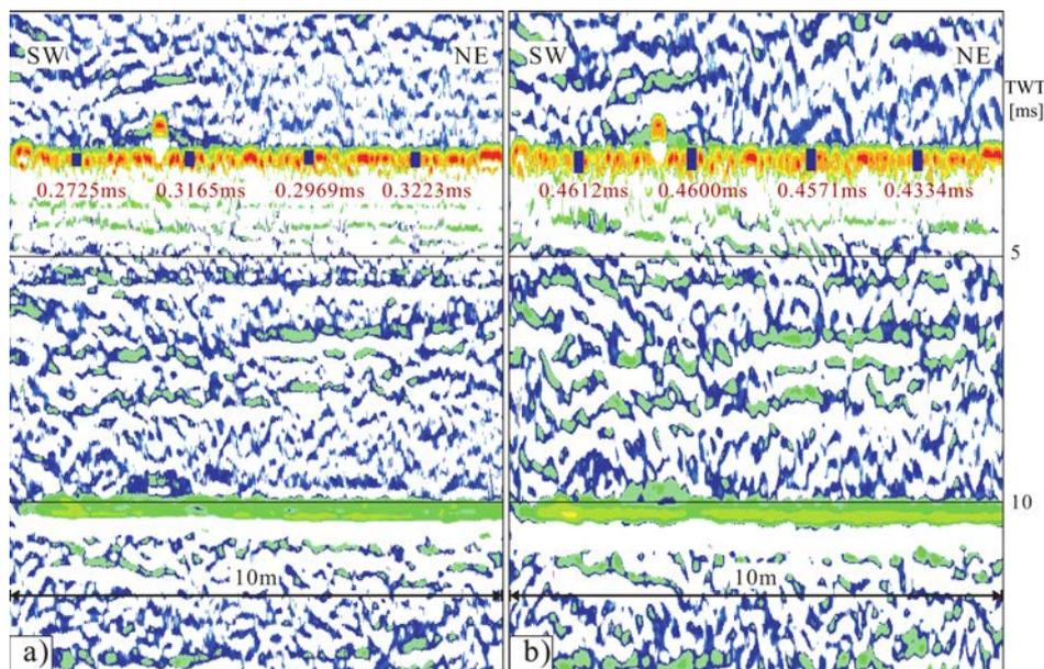
Fig. 7. Duration of the reflection event samples of SES-2000 SBP at 4 kHz: a) nominal PW was 250  $\mu\text{s}$ , measured resolution was 151.1  $\mu\text{s}$ , b) nominal PW was 500  $\mu\text{s}$ , measured resolution was 226.5  $\mu\text{s}$ .
