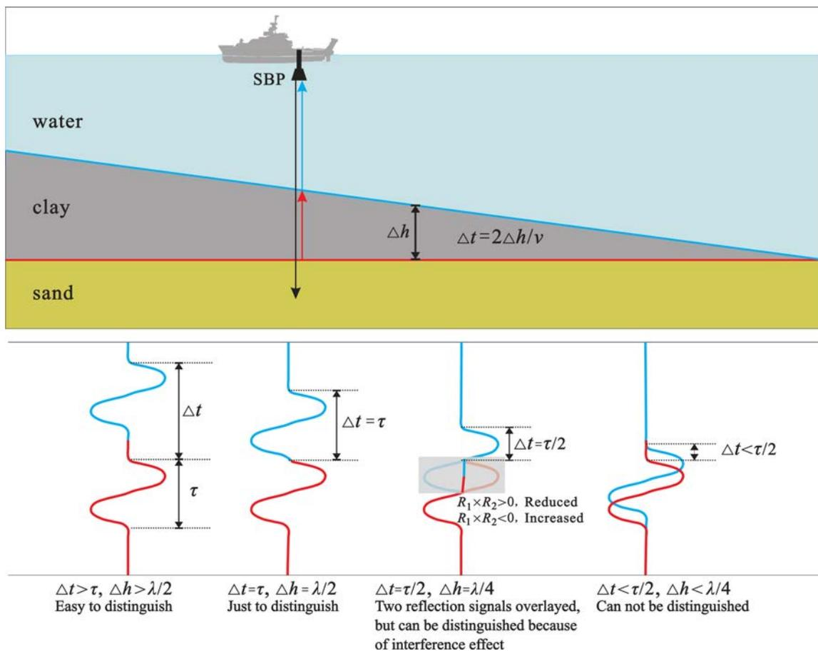
Fig. 1. Definition of the vertical resolution of SBP.  $\tau$  is the pulse width (PW),  $\Delta h = \lambda/2$ , the general vertical resolution, and  $\Delta h = \lambda/4$ , the extreme vertical resolution.
