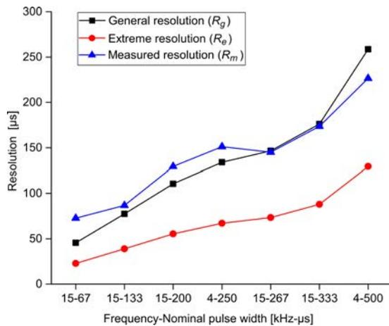
Fig. 9. Comparison of three kinds of vertical resolution of SES-2000 SBP. The measured resolution decreased with the increase of PW, close to the theoretical general resolution and far from the extreme resolution.
