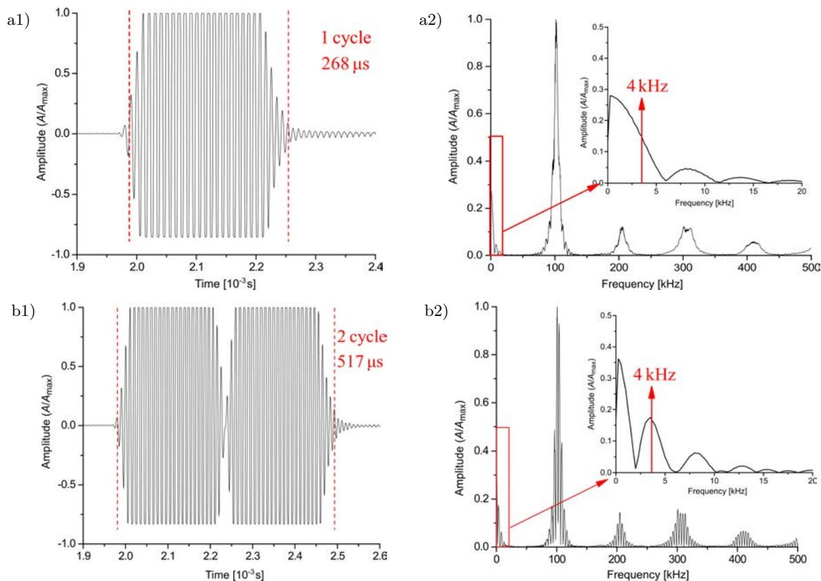
Fig. 3. Acoustic parameters measurement at 4 kHz setting: a1) was a time amplitude signal at 250  $\mu$ s PW setting, its measured PW was 268  $\mu$ s, and a2) was its frequency spectrum; b1) was a time amplitude signal at 500  $\mu$ s PW setting, its measured PW was 517  $\mu$ s, and b2) was its frequency spectrum.
