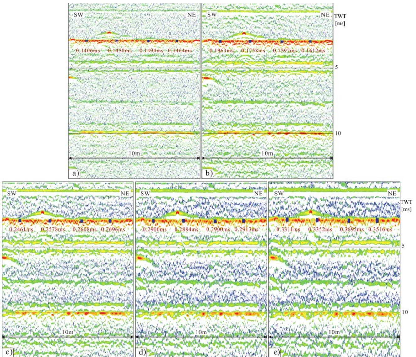
Fig. 8. Actual resolution samples of SES-2000 SBP at 15 kHz: a) nominal PW was 67  $\mu\text{s}$ , measured resolution was 72.7  $\mu\text{s}$ , b) nominal PW was 133  $\mu\text{s}$ , measured resolution was 86.7  $\mu\text{s}$ , c) nominal PW was 200  $\mu\text{s}$ , measured resolution was 129.3  $\mu\text{s}$ , d) nominal PW was 267  $\mu\text{s}$ , measured resolution was 145.0  $\mu\text{s}$ , e) nominal PW was 333  $\mu\text{s}$ , measured resolution was 173.5  $\mu\text{s}$ .
