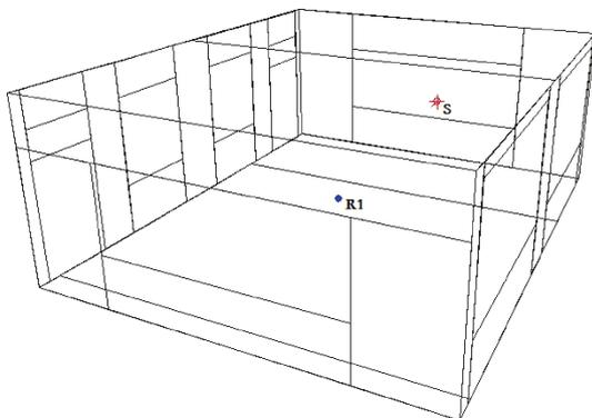
Fig. 1. The classroom model and the sound sources and listening positions in the model.
