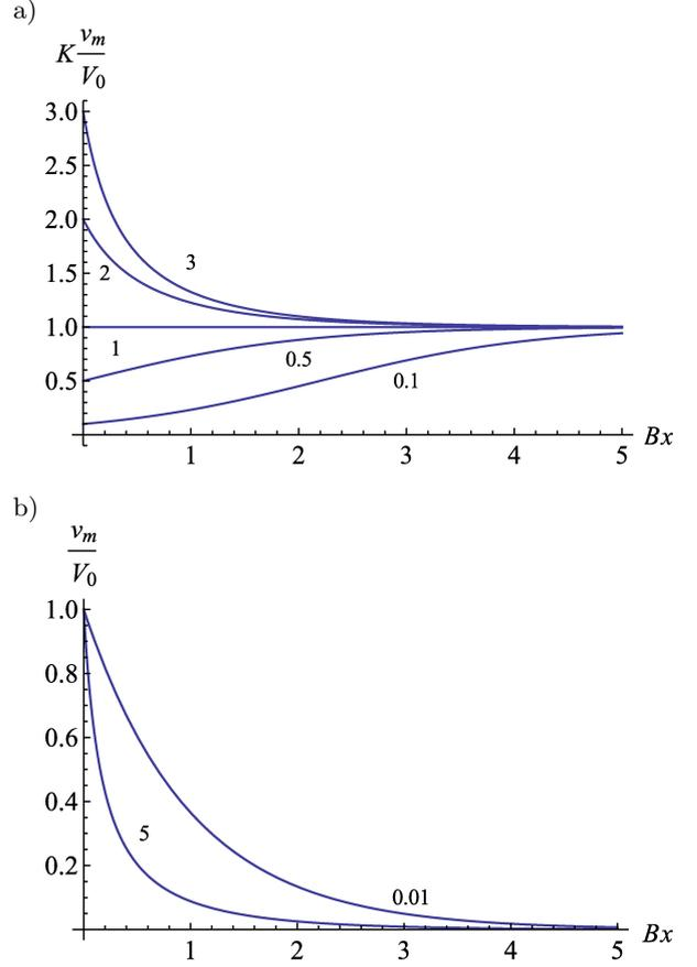
Fig. 2. Magnitude of a sawtooth impulse in the course of propagation as a function of dimensionless distance from a transducer. Cases of positive (a) and negative (b)  $B$ . The dimensionless quantity  $K = \frac{2\epsilon V_0}{BTc_m^2}$  which relates to every line stands by the correspondent curve.
