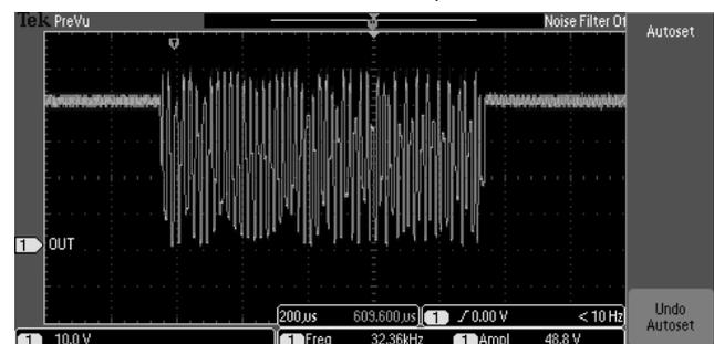
Fig. 3. The generated signal and its amplified version at the end of transmitting path.
