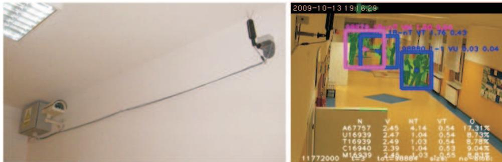
Fig. 4. One of the monitoring stations installed in a school (left), result of the motion analysis for the image acquired by the IP camera (right). Marked rectangles follow discovered “objects” in motion.
