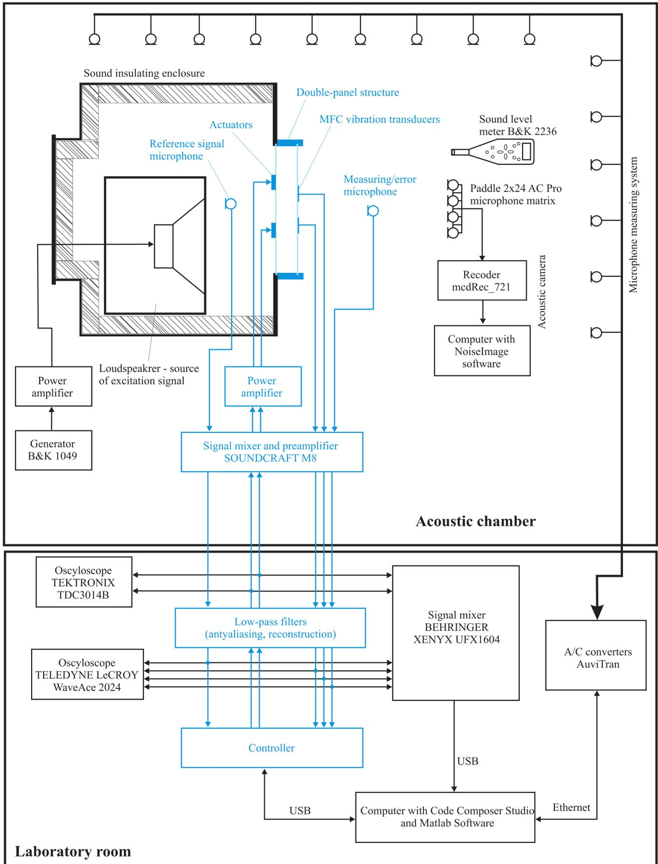
Fig. 4. Block diagram of the experimental setup.
