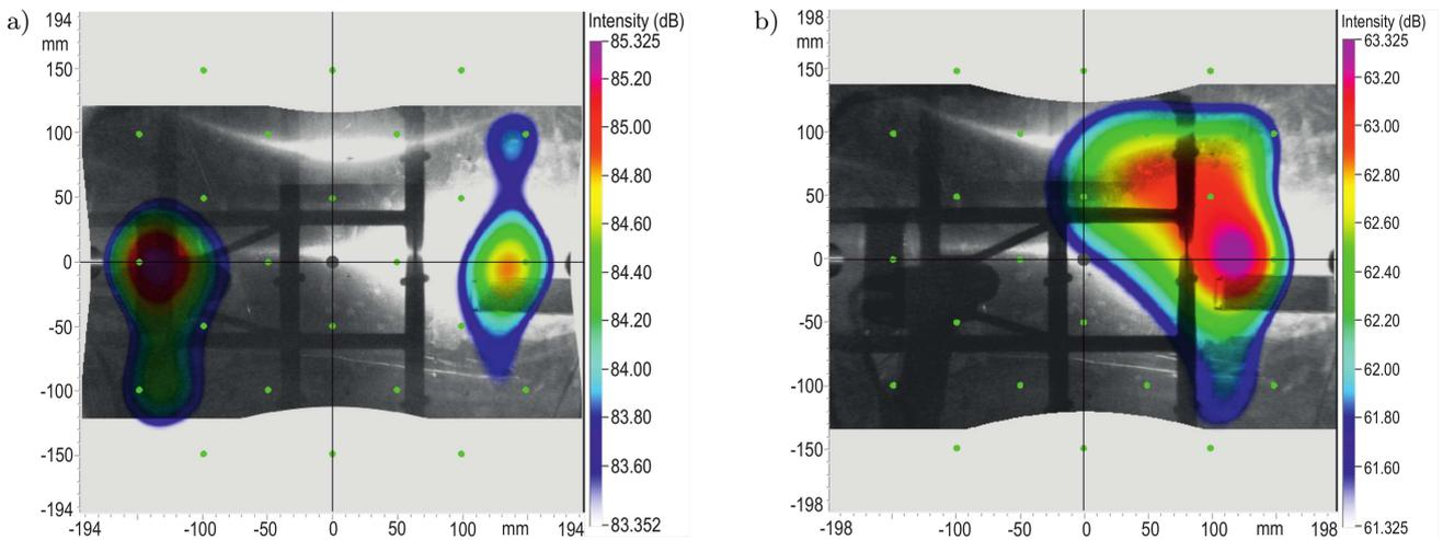
Fig. 6. Sound intensity levels and its distribution over the structure plate surface before (a) and after (b) ASAC system turned on.
