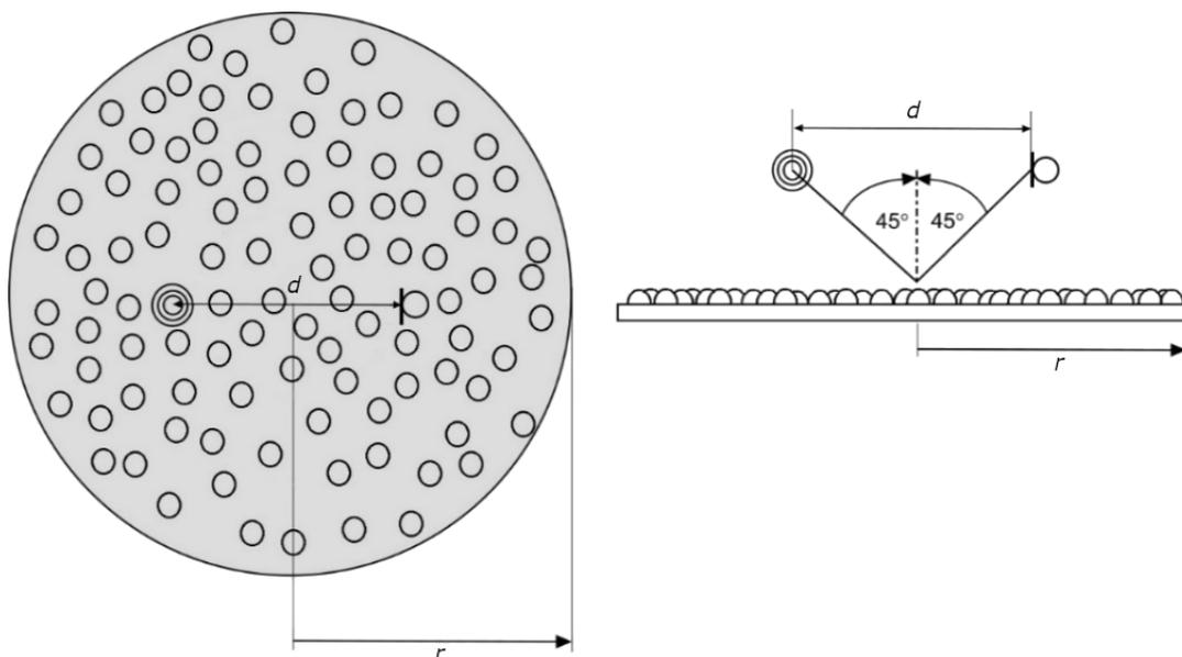
Fig. 4. Diffusing surface used for numerical and experimental tests. For the numerical tests  $r = 4.75$  m, scattering coefficient  $s$  from Table 4 was used. For the experimental tests the 1:10 scale model was used with  $r = 47.5$  cm, the disc was 50% covered with 4 cm wooden calottes.
