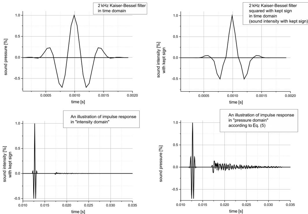
Fig. 3. Kaiser-Bessel filter 2 kHz octave band in time domain  $p_{KB}(t)$  (top left). Modified Kaiser-Bessel filter 2 kHz in the “intensity domain”  $I_{KB}(t)$ , according to Eq. (4) (top right). An illustration of impulse response in the “intensity domain” (bottom left). An illustration of impulse response in the “pressure domain” according to Eq. (5) (bottom right).
