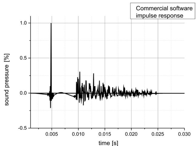
Fig. 10. Impulse response simulated with a commercial software.
