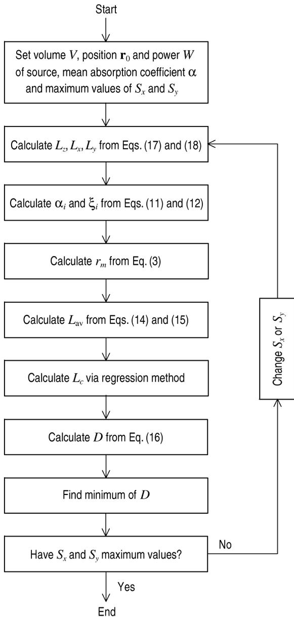
Fig. 2. Numerical procedure for finding optimum dimension ratios  $S_x$  and  $S_y$  for assumed input parameters: the room volume  $V$ , the position  $\mathbf{r}_0$  and the power  $W$  of the source and the mean absorption coefficient  $\alpha$ .
