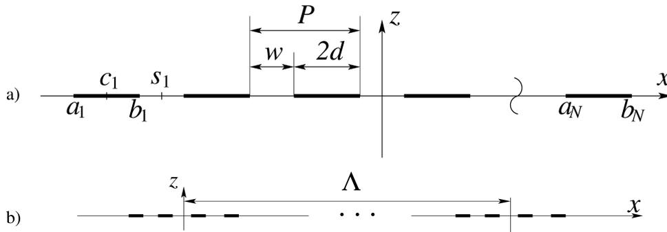
Fig. 1. a) A system of  $N$  rigid baffles (strips) on the boundary of acoustic media spanning for  $z > 0$ ; b) multi-periodic structure with certain large period  $\Lambda$  comprised by the replicas of the finite baffle system (a).
