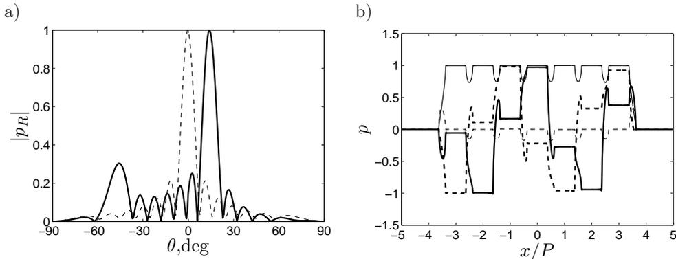
Fig. 2. a) Far-field radiation pattern for an 8 element baffle array; steering angle  $\beta = 15^\circ$  (a solid line) and  $\beta = 0^\circ$  (a dashed line);  $P = \lambda$ ,  $w = 0.75\lambda$ ; b) spatial distribution of  $p(x)$  on the baffle plane; steering angle  $\beta = 15^\circ$  (thick lines) and  $\beta = 0^\circ$  (a thin line); solid lines –  $\text{Re}(p)$ , dashed lines –  $\text{Im}(p)$ .
