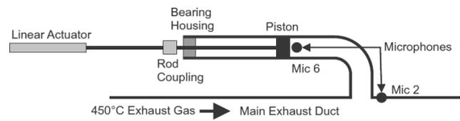
Fig. 12. Schematic view of the exhaust system and the adaptive quarter wave tube (HOWARD, CRAIG, 2014a).
