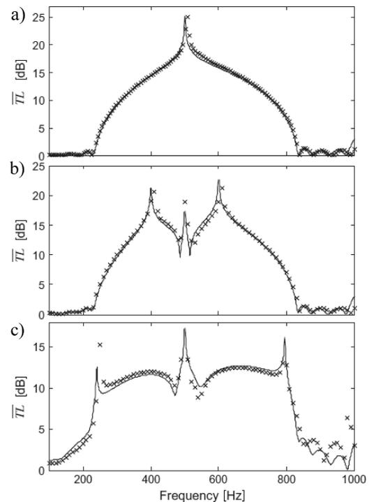
Fig. 4. Man made disorder in the geometries of Helmholtz resonators (x represents the FEM simulation and the solid lines represent the theoretical prediction): a)  $f_1 = f_2 = f_3 = f_4 = f_5 = 500$  Hz, b)  $f_1 = 400$  Hz,  $f_2 = 600$  Hz,  $f_3 = f_4 = f_5 = 500$  Hz, c)  $f_1 = 250$  Hz,  $f_2 = 800$  Hz,  $f_3 = f_4 = f_5 = 500$  Hz (WANG, MAK, 2014).
