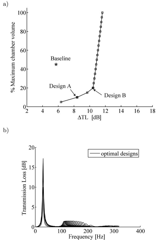
Fig. 8. Trade off curve with objective function adjusted to favour nominal desired frequency and constraint on diameter ratio (KURDI *et al.*, 2014).
