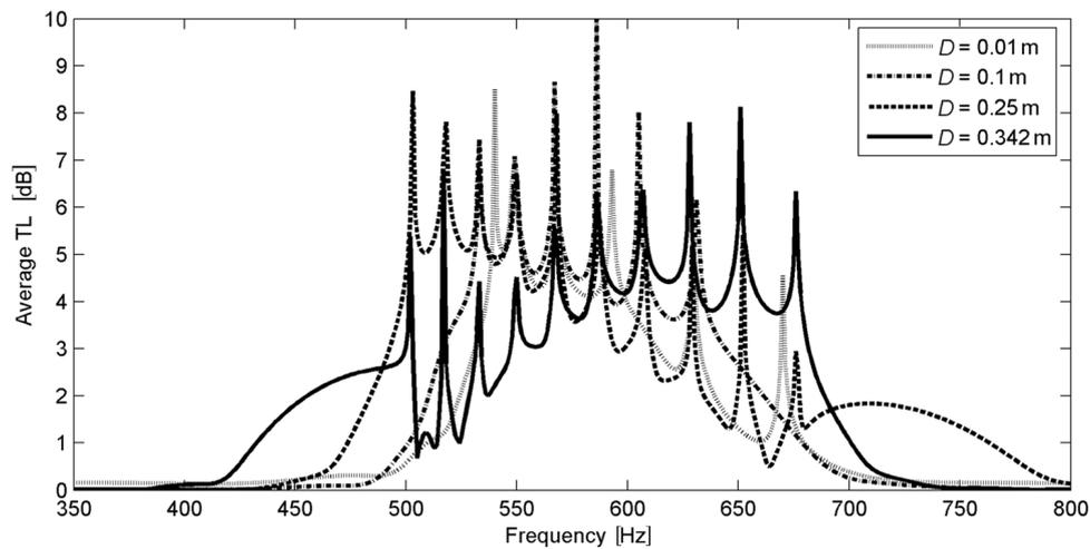
Fig. 11. Average TL of tubes of varying lengths with different periodic distance. Dotted line:  $D = 0.01$  m; dashed dotted line:  $D = 0.1$  m; dashed line:  $D = 0.25$  m; solid line:  $D = 0.342$  m (WANG *et al.*, 2016).
