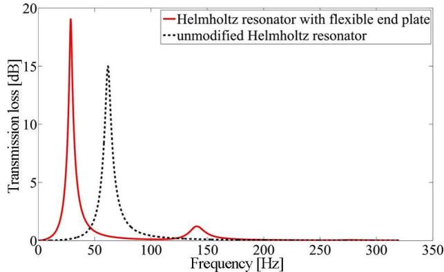
Fig. 7. Predicted transmission loss result (NUDEHI *et al.*, 2013).
