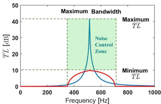
Fig. 5. Noise control zone for ducted HRs presented in the average TL curve (CAI, MAK, 2016).
