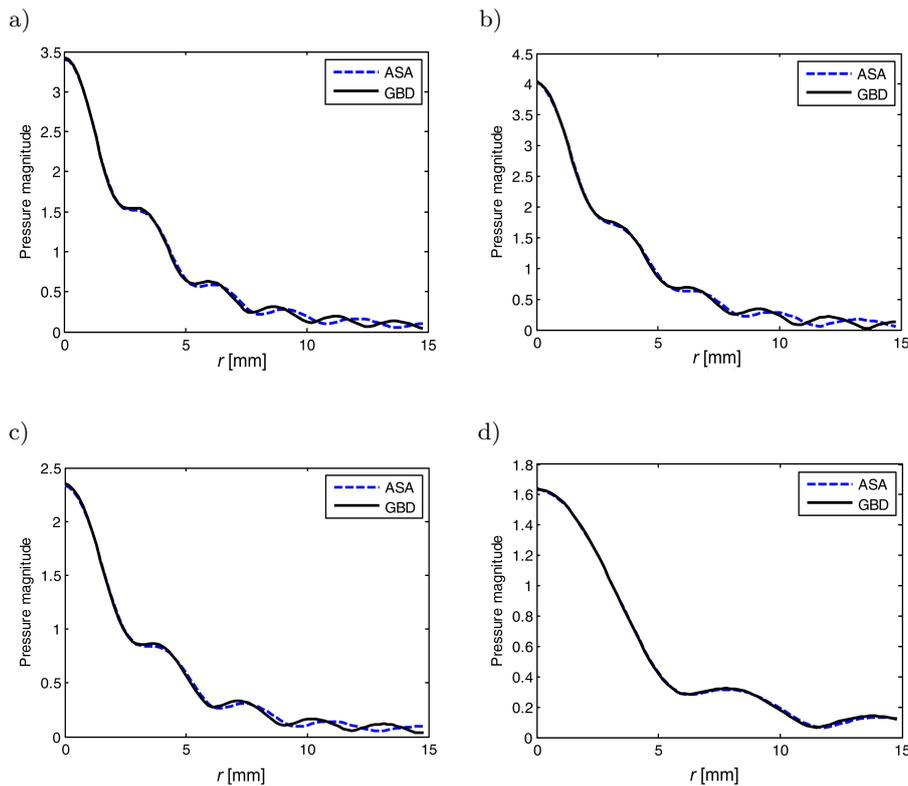
Fig. 3. Radial distributions of pressure. Incident field at  $z_1$  (a), internal field at  $z_f$  (b), and transmitted field at  $z_2$  (c) and at  $2z_f$  (d) (solid curve: GBD, dashed curve: ASA) for plexiglas plate.
