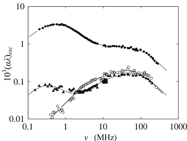
Fig. 13. Acoustical excess attenuation spectra at 25°C for 0.05 mol/l aqueous solutions of  $\alpha$ -cyclodextrin without ( $\circ$ ) and with  $n$ -octyl- $\beta$ -D-glucopyranoside ( $\blacktriangle$ , 0.016 mol/l  $\hat{=}$  0.44 cac;  $\bullet$ , 0.20 mol/l  $\hat{=}$  2.8 cac) added (HALLER, KAATZE, 2009c).
