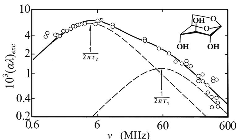
Fig. 3. Excess attenuation spectrum for an aqueous solution of 1,6-anhydro- $\beta$ -glucopyranoside (0.75 mol/l) and  $\text{Ca}(\text{ClO}_4)_2$  (0.77 mol/l) at 25°C. Dashed lines indicate the subdivision of the spectrum into two Debye-type relaxation terms with discrete relaxation times  $\tau_1$  and  $\tau_2$ , respectively. The full line represents the sum of these terms (COWMAN *et al.*, 1999).
