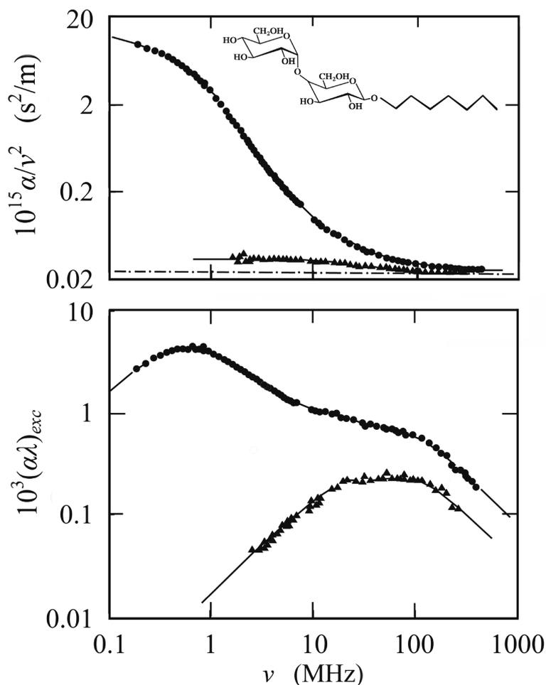
Fig. 6. Acoustical attenuation spectra in the frequency normalized format (top) and as excess attenuation per wavelength (bottom) for two aqueous solutions of *n*-hexyl- $\beta$ -D-maltopyranoside at 25°C (cmc = 0.201 mol/l):  $\blacktriangle$ ,  $c = 0.150$  mol/l;  $\bullet$ ,  $c = 0.225$  mol/l (HALLER, KAATZE, 2009b).
