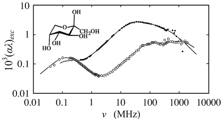
Fig. 2. Acoustical excess attenuation spectra for solutions of 0.5 mol/l D-fructose in water at 25°C without (○) and with (●)  $\text{CaCl}_2$  added (BAUCKE *et al.*, 2004a). The salt concentration is 0.5 mol/l.
