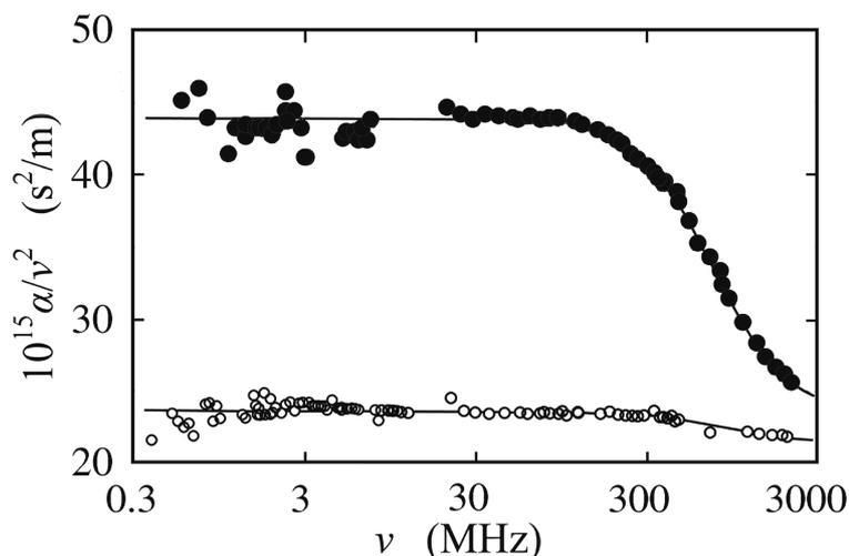
Fig. 1. Acoustical attenuation coefficient  $\alpha$  per  $\nu^2$  versus frequency  $\nu$  for 1 mol/l solutions of calcium nitrate (●) and calcium chloride (○) in water at 25°C (BAUCKE *et al.*, 2004b).
