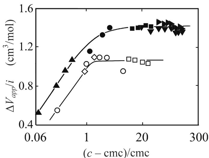
Fig. 10. Lin-log plot of the apparent reaction volume per methylene group,  $\Delta V_{\text{app}}/i$ , versus reduced concentration,  $c/\text{cmc}-1$ , for alkyl glucoside (open symbols) and alkyl maltoside (filled symbols) solutions at 25°C (HALLER, KAATZE, 2009b). See Fig. 7 for the figure symbols.
