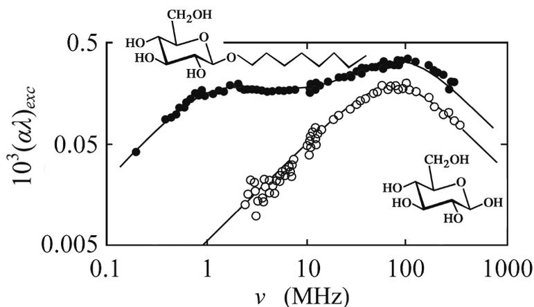
Fig. 5. Acoustical excess attenuation spectra for aqueous solutions of *n*-hexyl- $\beta$ -D-glucopyranoside (●, cmc = 0.25 mol/l) and of D-glucose (○) at 25°C (HALLER, KAATZE, 2009a). With both spectra the solute concentration is 0.2 mol/l.
