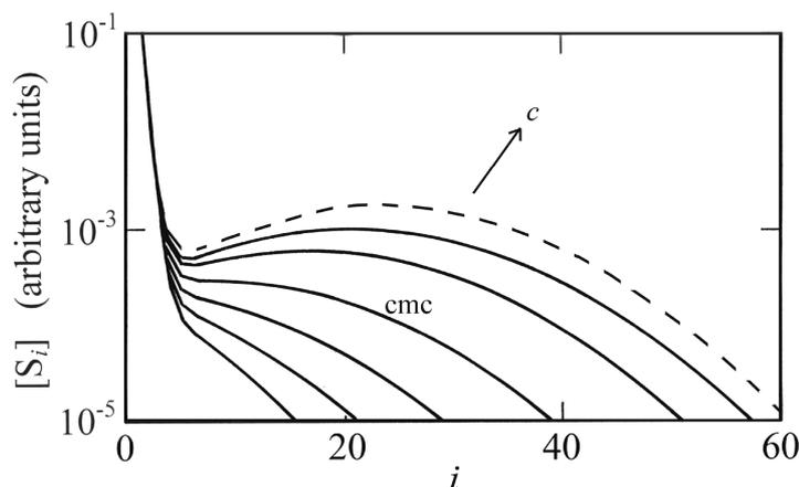
Fig. 15. Logarithmic plot of concentrations  $[S_i]$  of aggregates containing  $i$  monomers *versus* aggregation number  $i$  with surfactant concentration  $c$  as a parameter: results from model calculations of an extended Teubner-Kahlweit theory (TELGMANN, KAATZE, 1997a).
