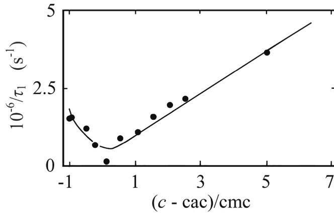
Fig. 14. Relaxation rate  $\tau_1^{-1}$  of relaxation term due to surfactant monomer exchange in the micelle formation/disintegration kinetics *versus* scaled concentration  $(c - cac)/cmc$  for aqueous solutions of  $C_8G_1$  and CD ( $c(CD) = 0.05$  mol/l;  $c = [C_8G_1]$ ; 25°C).
