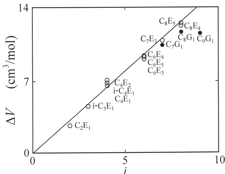
Fig. 9. Reaction volume as following from Eq. (8),  $\Delta V$ , versus number of methyl/methylene groups per alkyl chain,  $i$ , for solutions of alkyl glucosides ( $\bullet$ ,  $C_iG_1$ ; HALLER, KAAATZE, 2009a) and poly(ethylene glycol) monoalkyl ethers ( $\circ$ ,  $\text{CH}_3(\text{CH}_2)_{i-1}(\text{OCH}_2\text{CH}_2)_j\text{OH}$ ,  $C_iE_j$ ; TELGMANN, KAAATZE, 2000a; 2000b). Only the largest values of concentration series are shown, respectively.
