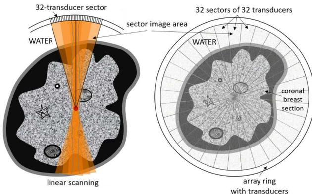
Fig. 1. The linear echographic scanning of the breast *in vivo* using fragments (sections of multiple transducers) of the ring array, with natural focusing on the axis of the transducer ring: a) the method of obtaining an image from a single section, b) diagram showing the combination of the cross-section of the breast from all sections.
