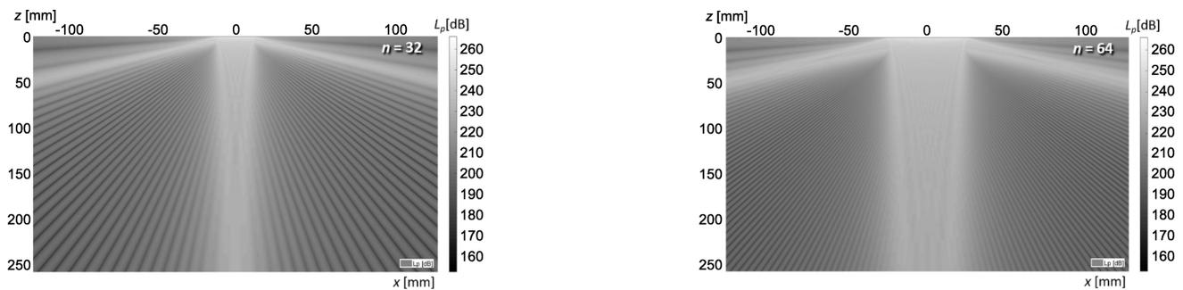
Fig. 11. Results of the acoustic field distribution  $L_p(x, 0, z)$  for sectors of the linear array with the number of activated transducers  $n = 32$  and  $n = 64$ , in the form of black-and-white graphs.
