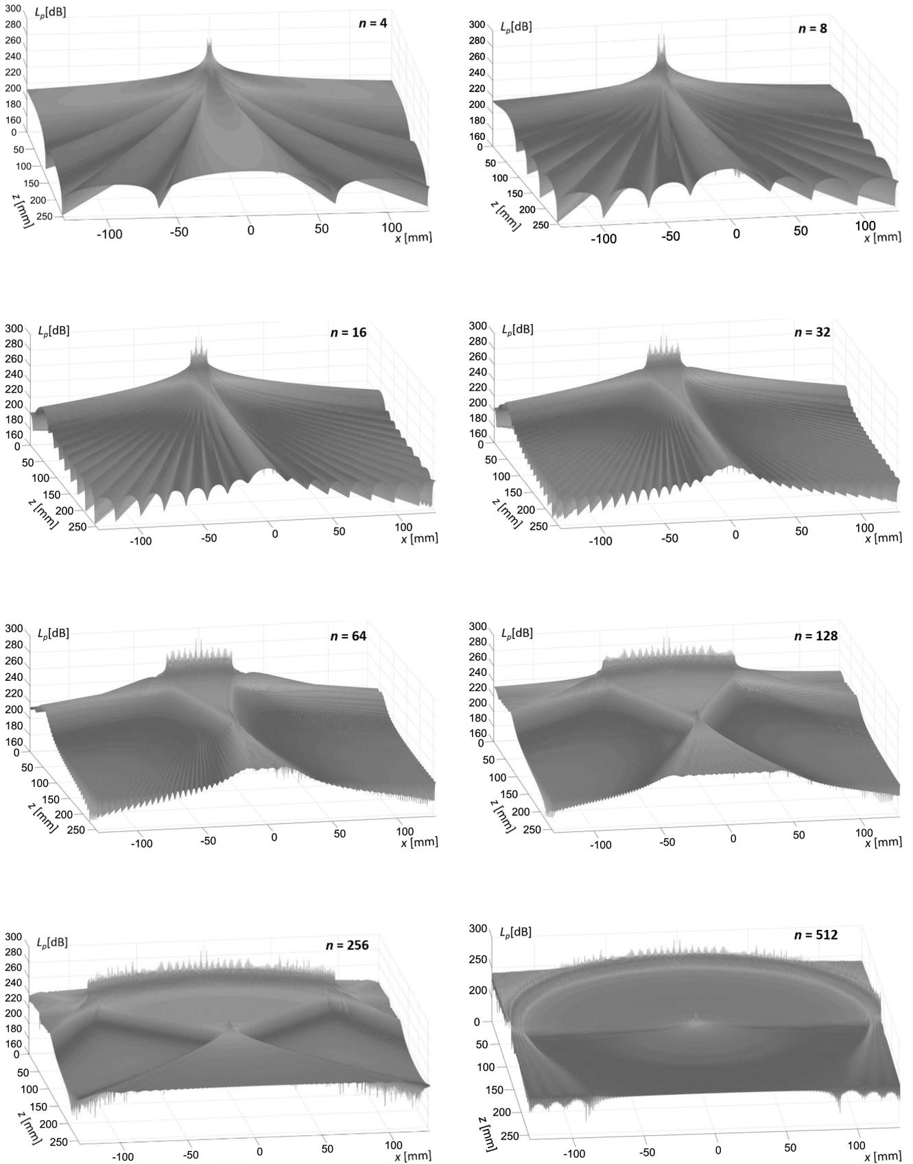
Fig. 6. The results of the acoustic field distribution calculations in the form of  $L_p(x, 0, z)$  for sectors of the ring array with varying numbers of activated transducers ( $n = 4, 8, 16, 32, 64, 128, 256, 512$ ), in the form of pseudo-three-dimensional graphs.
