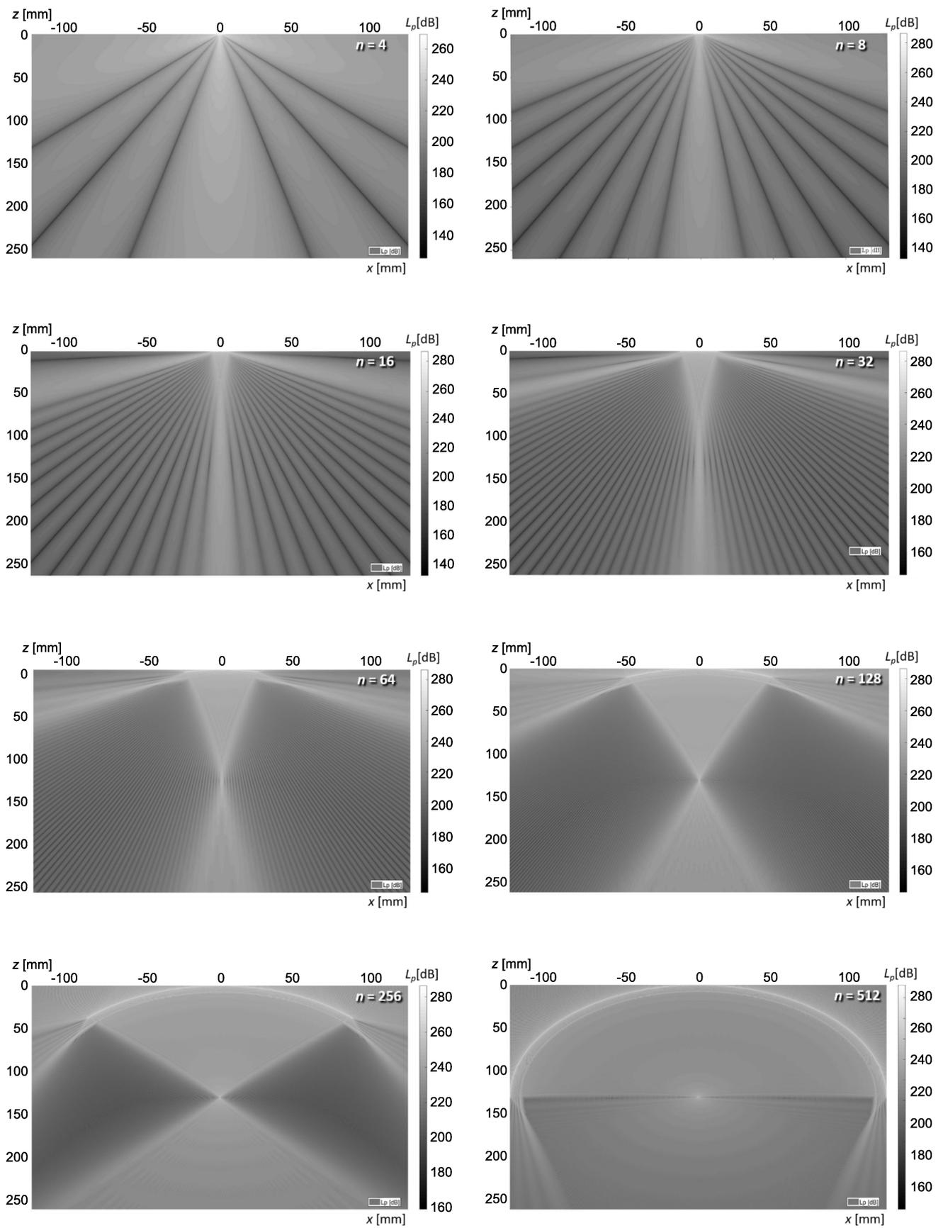
Fig. 7. Results of the acoustic field distribution calculations in the form of  $L_p(x, 0, z)$  for sectors of the ring array with varying numbers of activated transducers ( $n = 4, 8, 16, 32, 64, 128, 256, 512$ ), in the form of black-and-white graphs.
