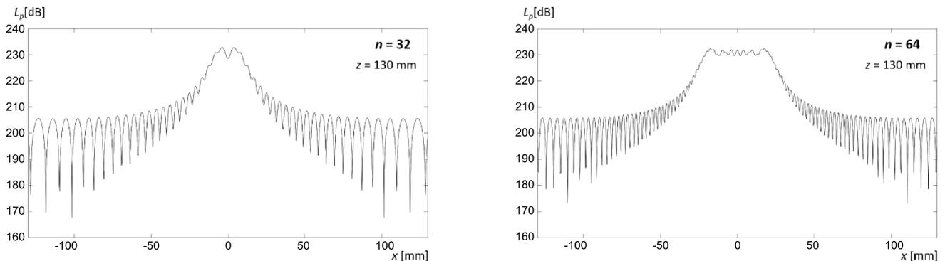
Fig. 12. Results of the acoustic field distribution  $L_p(x)$  for  $y = 0, z = 130$  mm, for sectors with the number of activated transducers  $n = 32$  and  $n = 64$ , in the form of linear distribution graphs.
