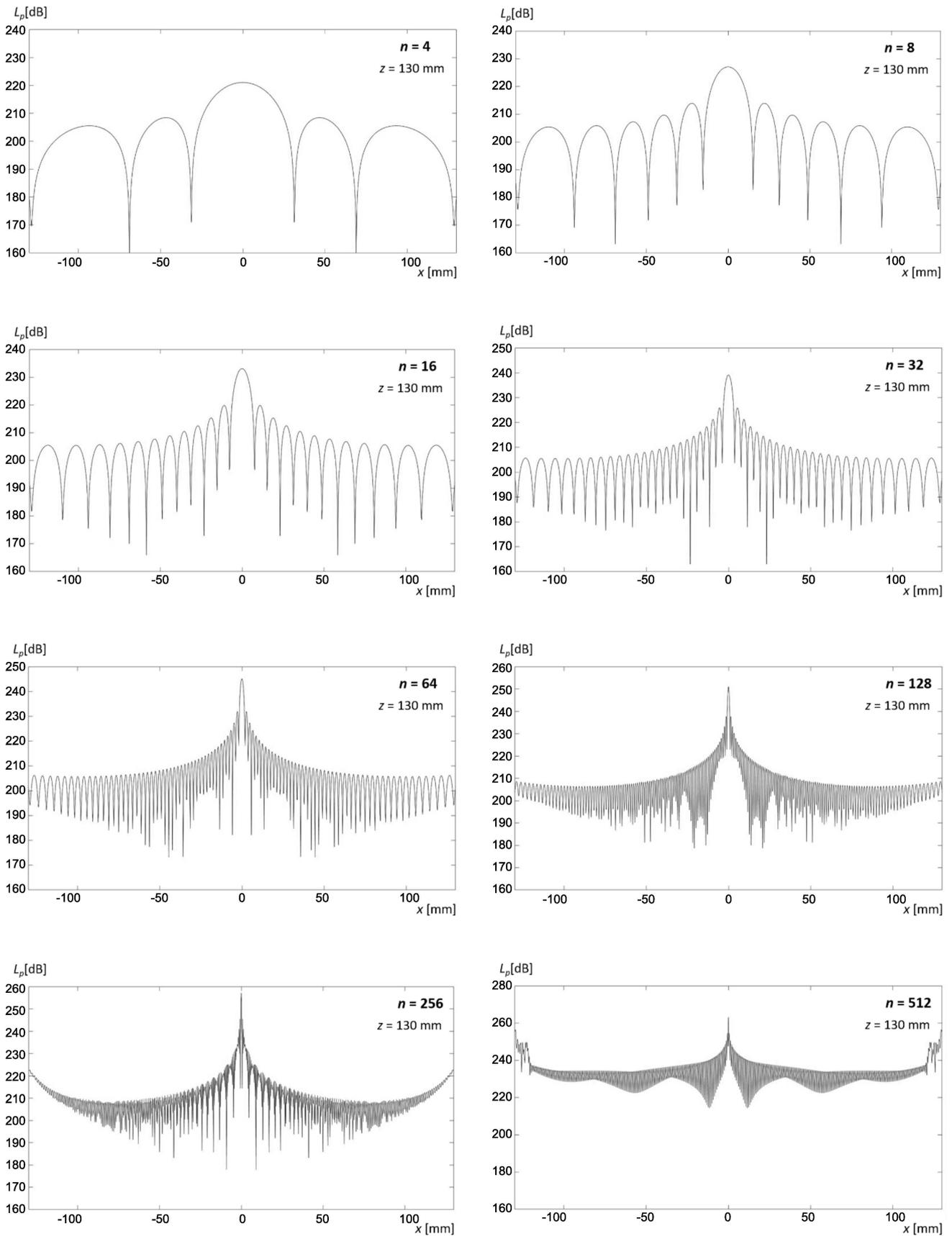
Fig. 8. Results of the acoustic field distribution calculations  $L_p(x)$  for  $y = 0$ , on diameter of the ring array ( $z = R_p = 130$  mm), for sectors of the ring array with varying numbers of activated transducers ( $n = 4, 8, 16, 32, 64, 128, 256, 512$ ), in the form of linear distribution graphs.
