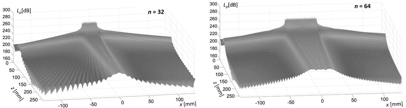
Fig. 10. Results of the acoustic field distribution  $L_p(x, 0, z)$  for sectors of the linear array with the number of activated transducers  $n = 32$  and  $n = 64$ , in the form of pseudo-three-dimensional graphs.
