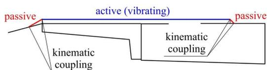
Fig. 3. Fixation of strings in numerical model.
