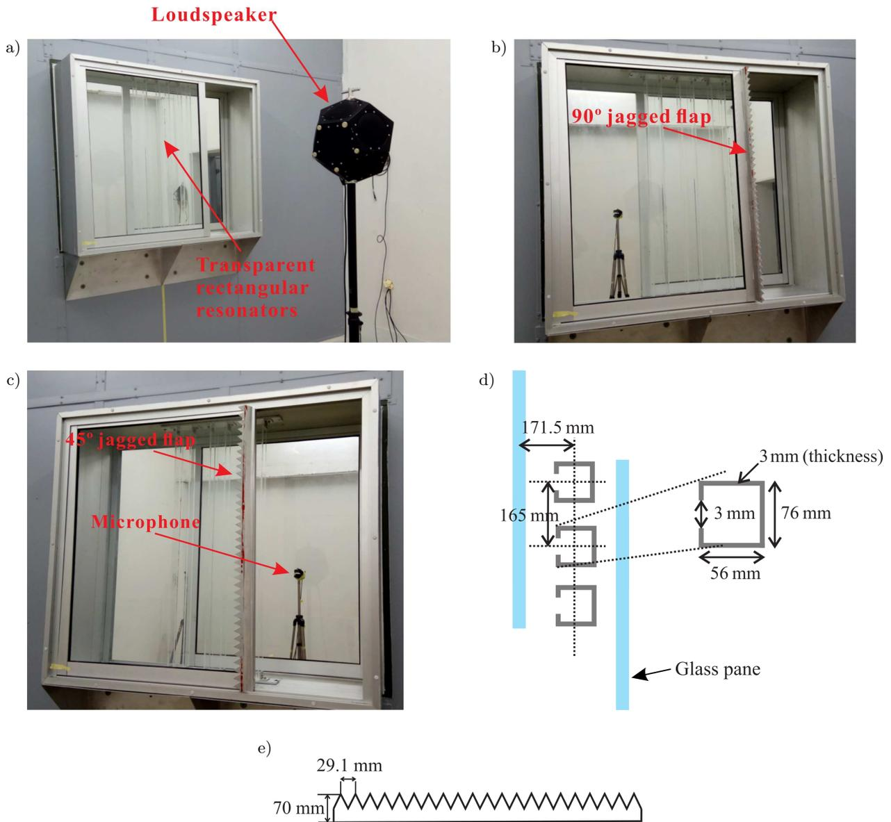
Fig. 1. a) Experimental set-up of the plenum window with rectangular HRs at reverberation room, b) plenum window with attached 90° jagged flap, c) plenum window with attached 45° jagged flap, d) geometry of the plenum window with HRs (top view), e) geometry of the jagged flap.
