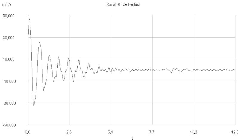
Fig. 7. The time courses of the vibration velocity of the bridge: a) before and b) after the installation of TMD.
