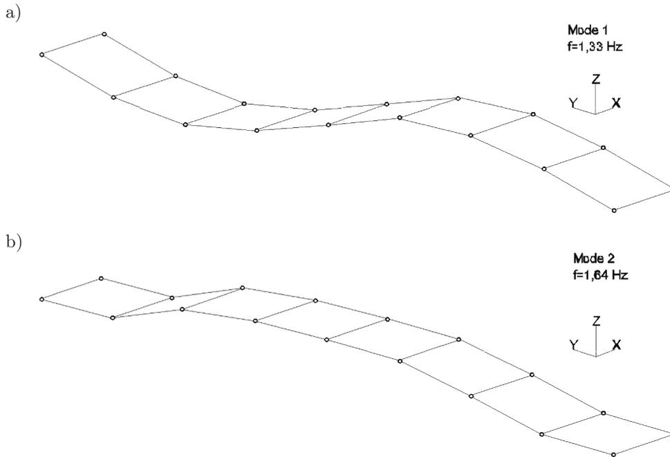
Fig. 4. The results of modal analysis, the measured figures of vibrations at frequencies:
