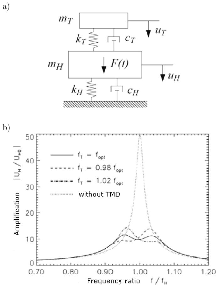
Fig. 2. The two mass system a) and b) amplification function for several tuning frequencies.
