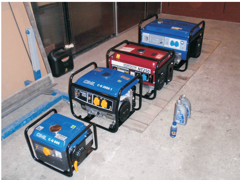
Fig. 3. Gasoline engine-generators prepared for acoustic measurements.
