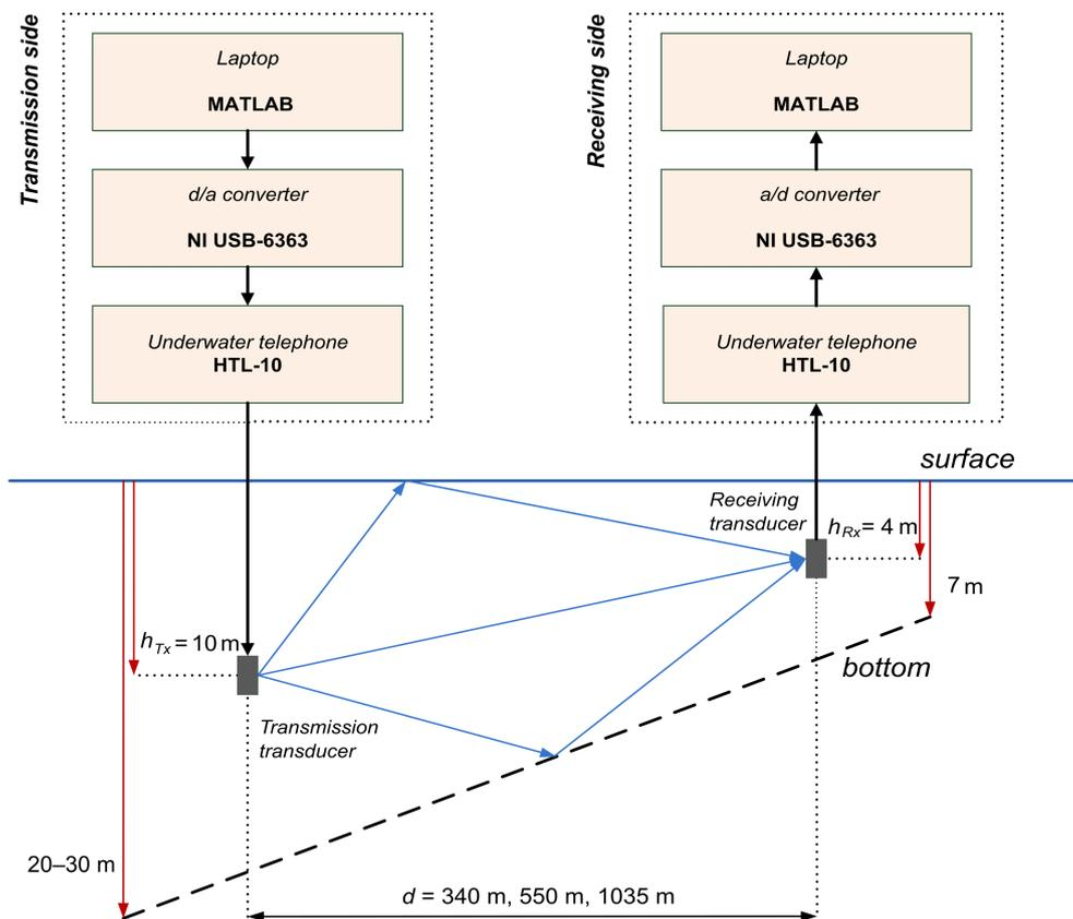
Fig. 3. Measuring system.
